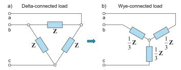
Fig. 11.27. Delta-connected load versus ad.
