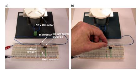
Fig. 18.26. MOSFET actuator circuit with a temperature sensor and a 12-V DC motor.
