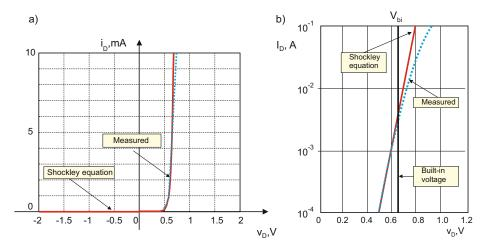
Fig. 16.4. (a) Shockley equation prediction (*solid curve*) versus measured data (*dotted curve*) for the 1N4148 small-signal Si switching diode at 25  $^{\circ}$ C and (b) enlarged scale.
