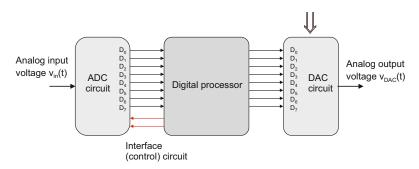
Fig. 14.14. Place of the DAC in the DSP block diagram.
