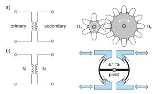
Fig. 12.5. Analogies for a transformer.
