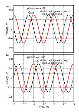
Fig. 8.2. Phase-shifted AC voltages  $v(t) = 0.6 \cos (2\pi 1000t \pm \pi/2)$  [V] versus the zero-phase voltage  $v(t) = 0.6 \cos (2\pi 1000t)$  [V] shown by a *solid curve*. In Fig. 8.2a the *dashed* voltage leads the base signal, whereas in Fig. 8.2b it lags the base signal.
