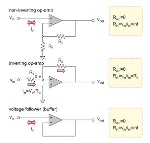
Fig. 5.18. Input and output resistances of amplifier circuits with the ideal operational amplifier.
