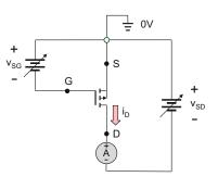
Fig. 18.15. Schematic diagram of the PMOS transistor test circuit.
