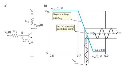
Fig. 17.33. BJT common-emitter amplifier and its simplified voltage transfer characteristic.
