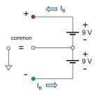
Fig. 3.9. A dual-polarity power supply constructed with two battery cells.
