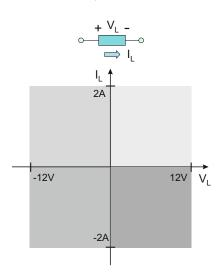
**Problem 13.14.** In a switching circuit shown in the figure that follows, an IRF510 n-channel power MOSFET with  $V_{\text{Tn}} = 3.5$  V is used. Assuming zero switch resistance, determine the power delivered to the load when the control voltage is:
