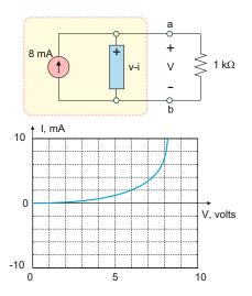
**Problem 4.67.** A circuit shown in the following figure contains a nonlinear passive element. The *v*-*i* characteristic of the nonlinear element (the ideal Shockley diode) is
