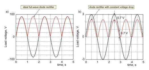
Fig. 16.23. Rectified (or load) voltage versus source voltage. (a) The result for the ideal full-wave diode rectifier or full-wave rectifier with a high input signal. (b) The result using the constant-voltage-drop-diode model for a moderate input signal.
