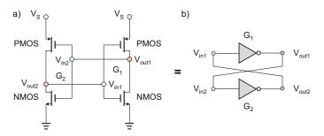
Fig. 13.32. Basic latch consisting of two inverters.
