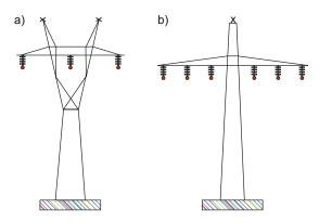
Fig. 11.21. (a) Three-phase single-circuit high-voltage overhead power transmission line and (b) three-phase double-circuit, high-voltage overhead line. Both lines include (thinner) shielding wire (s) on top of it to protect against lightning strikes (F. Kiessling, et al., "*Overhead Power Lines: Planning, Design, Construction*," Springer 2003).
