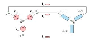
Fig. 11.22. Three-phase balanced wye-wye system with the neutral conductor removed. The neutral conductor may still be implied for the solution using the per-phase method.
