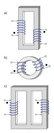
**Problem 12.3.** For the circuit shown in the following figure, determine voltage  $v_2(t)$  if  $v(t) = 100 \cos \omega t$  [V] using Faraday's law of induction. Count the number of turns. Assume no flux leakage.
