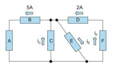
**Problem 3.8.** Find currents  $i_A$ ,  $i_B$ ,  $i_D$ ,  $i_H$  for the circuit shown in the following figure:
