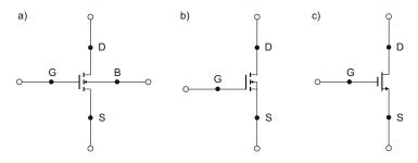
Fig. 18.2. Circuit symbols of (a) a four-terminal NMOS transistor, (b) a three-terminal asymmetric NMOS transistor with the body tied to the source, and (c) the same device but simplified.
