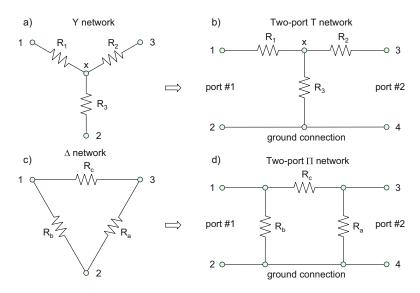
Fig. 3.29. Conversion of Y and  $\Delta$  three-terminal networks to equivalent T and  $\Pi$  two-port, four-terminal networks.
