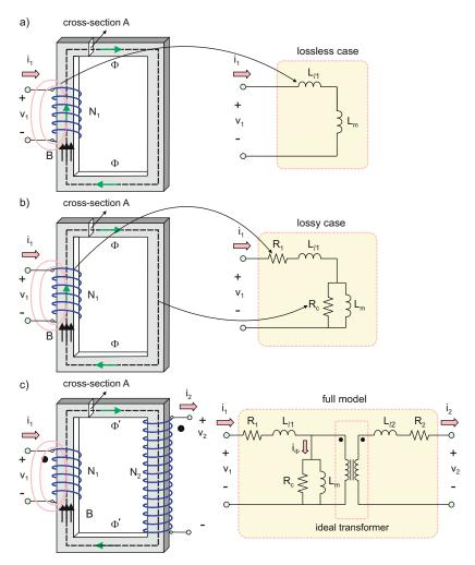
Fig. 12.16. Circuit model of a low-frequency transformer—the Steinmetz model.
