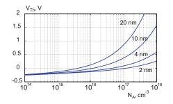
Fig. 18.7. Threshold voltage as a function of  $N_A$  and  $t_{OX}$  (Al gate).
