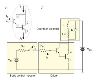
Fig. 17.31. Automotive door lock solenoid driven by Darlington pair.
