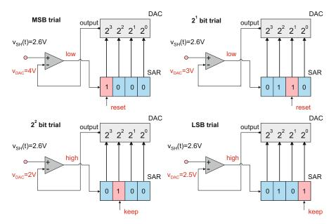
Fig. 14.28. Operation of a 4-bit successive-approximation ADC.
