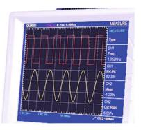
Fig. 8.4. Front panel of an inexpensive dual-channel digital-storage oscilloscope. Note the measured signal parameters.
