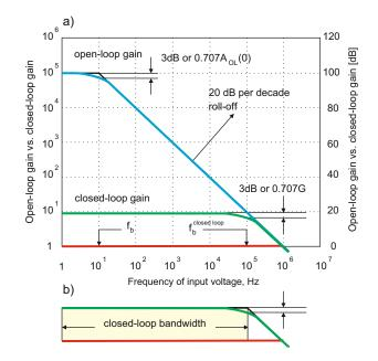
Fig. 9.13. Closed-loop AC gain  $A_{CL}(f)$  (*lower curve*) versus open-loop AC gain  $A_{OL}(f)$  (*upper curve*) for an inverting amplifier with  $A_{OL}(0) = 10^5$  and  $1 + R_2/R_1 = 10$  (the amplifier DC gain is -9).
