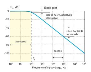
Fig. 9.4. Construction of a Bode plot for the amplitude transfer function of a low-pass RC filter with break frequency of  $f_{\rm b} = 100$  Hz.
