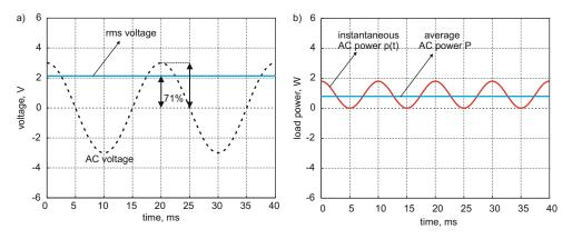
Fig. 11.2. (a) Load voltage  $v(t) = 3 \cos(2\pi 50t)$  [V] (*dotted line*) and its *rms* DC voltage, which delivers the same power into the load and (b) instantaneous power and the average power for the load voltage  $v(t) = 3 \cos(2\pi 50t)$  [V].
