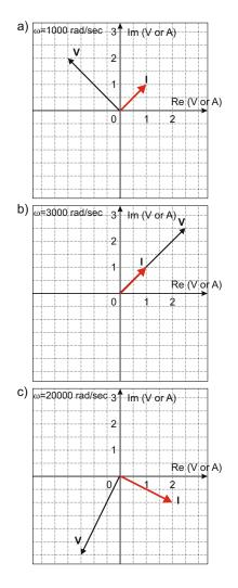
**Problem 8.47.** Phasor voltages and phasor currents for three unknown circuit elements are shown in the figure below. Determine the type of the element (R, L, or C) and the value of R, L, or C when appropriate.
