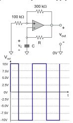
Sketch to scale the capacitor voltage,  $v_C$ , as a function of time. Assume that  $v_C(t = 0) = 0$ . Assume the ideal amplifier model. The specific values of *R* and *C* do not matter; they are already included in the time scale.
