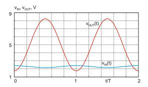
Fig. 18.31. Input and output voltages for the common-source amplifier from Example 18.10.
