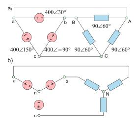
**Problem 11.54.** A balanced delta-delta system shown in the figure below operates at 50 Hz. The phase voltages of the delta source,  $V_{ab}$ ,  $V_{bc}$ ,  $V_{ca}$ , have the amplitudes of  $V_m = 563.4$  V each. Every phase impedance is a 0.21 H inductance in series with a 38- $\Omega$  resistance:
