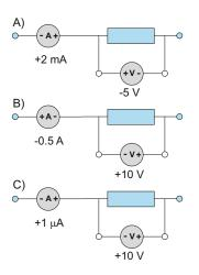
Based on voltage and current measurements, determine if the element is a resistance or a current source. Then, find the power delivered to the circuit element or taken from it in every case.
