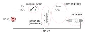
Fig. 7.15. Modeling the ignition system as in a laboratory. The spark plug voltage is about 3–10 kV.
