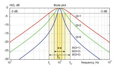
Fig. 10.5. Amplitude of the circuit current (or the amplitude of the resistor voltage) normalized by its peak value at resonance. The resulting graph is the Bode plot.
