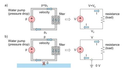
Fig. 2.36. A large reservoir at atmospheric pressure attached to a pumping system serves as an analogy to the ground connection in an electric circuit.
