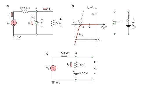
Fig. 16.19. (a) Shunt voltage regulator on the base of a Zener diode. (b). Piecewise-linear diode model for the Zener diode in the breakdown region. (c) The circuit from (a) with the Zener diode replaced by its equivalent circuit and with the open-circuited load.
