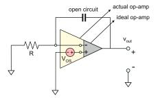
Fig. 6.25. Effect of the input offset voltage on the integrator circuit at DC.
