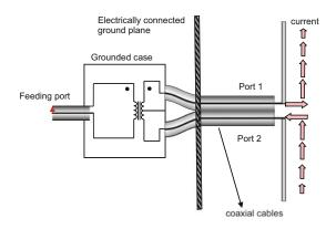
Fig. 12.14. A balun (center-tapped) transformer attached to a dipole antenna. The metal case of the transformer is grounded.
