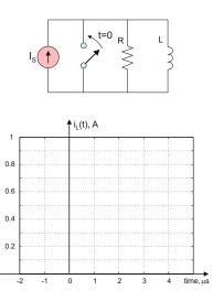
**Problem 7.36.** A 270- $\mu$ H inductor, shown in the following figure, releases its energy into the 510- $\Omega$  load resistor. The supply current is 0.8 A.
