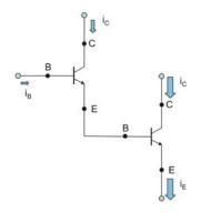
**Problem 17.7.** An npn-junction transistor in the active region at room temperature of 25 °C has  $v_{\rm BE} = 0.5 \text{ V}, I_{\rm S} = 10^{-13} \text{ A}$ , and the base current of 0.3  $\mu$ A. Find collector current, emitter current, common-emitter current gain, and common-base current gain. Show units.
