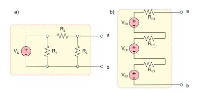
Fig. 4.13. Two active linear networks.
