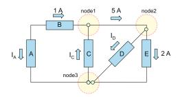
Fig. 3.3. Solving in a network using KCL.
