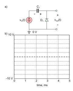
**Problem 16.66.** In the clamper circuit shown in the figure for Problem 16.65,  $v_{in}(t) = V_m - V_m \sin \omega t$  and  $V_m = 4$  V. The wave period is 2 ms.
