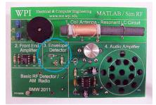
Fig. 16.28. AM radio receiver circuit with the envelope detector.
