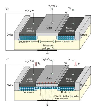
Fig. 18.4. Simplified NMOS configuration and creating a channel for current flow.
