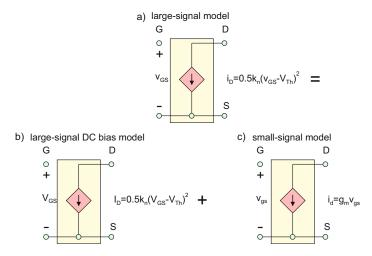
Fig. 18.29. Splitting the large-signal MOSFET model into a large-signal DC model and a small-signal model. This consideration applies to the common-source amplifier and to other circuits.
