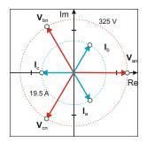
Fig. 11.23. Phasor diagram for the three-phase circuit of Example 11.11. Note the separate scales for the phasors of voltages and phasors of currents.
