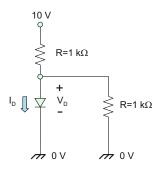
**Problem 16.20.** For the diode circuit shown in the following figure, determine the values of the diode current and the voltage across the diode, assuming that the diode is ideal.
