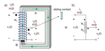
Fig. 12.10. Step-down autotransformer along with the corresponding circuit symbol. Circuit symbols for the autotransformer may vary.
