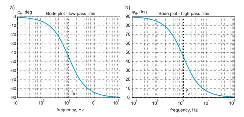
Fig. 9.6. Comparison of the phase Bode plots for (a) the low-pass-filter and (b) for the high-pass filter with the same break frequency  $f_{\rm b} = 1\,$  kHz. Both plots are identical to within a phase shift.
