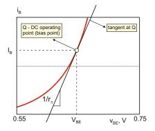
Fig. 17.34. Finding the small-signal base-emitter amplifier resistance  $r_{\pi}$ .
