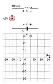
**Problem 10.4.** For a series ideal LC circuit shown in the figure below, the voltage source has the form  $v_{\rm S}(t) = V_{\rm m} \cos \omega t$ . Given  $V_{\rm m} = 5$  V, L = 1 mH,  $C = 0.5 \mu$ F:
