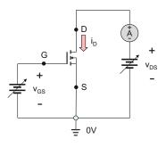
Fig. 18.11. Schematic diagram of the NMOS transistor test circuit.
