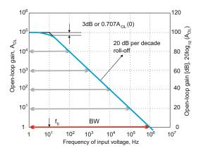
Fig. 9.11. Bode plot of the open-loop gain magnitude for the LM741-type amplifier IC. Note the logarithmic scale on the *left* and the corresponding scale in dB on the *right*. The frequency bandwidth given by the break frequency  $f_b$  is only 10 Hz.
