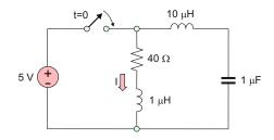
Fig. 6.17. A circuit is used to study the DC steady state. The switch closes at t = 0. The behavior of the circuit at  $t \to \infty$  is sought after the circuit has stabilized.
