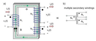
Fig. 12.11. A multiwinding transformer along with the corresponding circuit symbol. Circuit symbols for the multiwinding transformer may vary.
