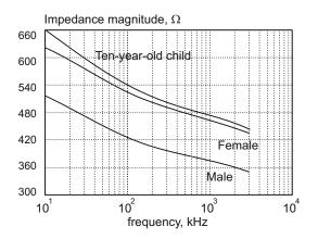
Fig. 8.13. Magnitude of the average impedance of the human body. From: I. Chatterjee et al., "Human Body Impedance and Threshold Currents for Perception and Pain for Contact Hazard Analysis in the VLF-MF Band," *IEEE Trans Biomedical Eng.*, May 1986.
