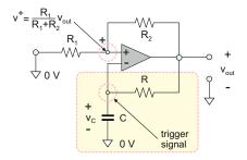
Fig. 7.19. Bistable amplifier circuit with an RC circuit in the negative feedback loop.
