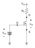
**Problem 18.41.** A solution for an unknown fixed-gate circuit shown in the previous problem is given in the figure that follows. Restore the transistor and circuit parameters (show units):
