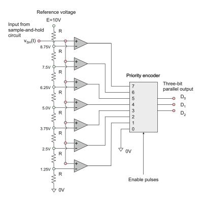
Fig. 14.26. A 3-bit flash ADC.
