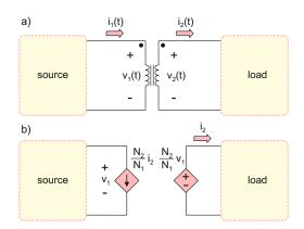
Fig. 12.3. Transformer interfacing a source and a load and its model in terms of dependent sources.
