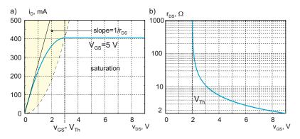
Fig. 18.18. MOSFET turn-on resistance  $r_{DS}$  and its dependence on gate-source voltage for a 2 N7000 NMOS device.
