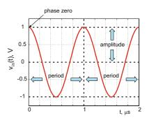
Fig. 14.21. Analog continuous voltage in the form of a cosine function.
