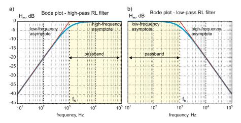
Fig. 9.10. (a) Bode plot for the amplitude transfer function of the high-pass RL filter with break frequency  $f_{\rm b} = 1$  kHz. (b) The same Bode plot but for the low-pass RL filter.
