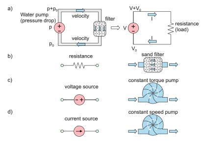
Fig. 1.9. Hydraulic analogies in the DC steady state.
