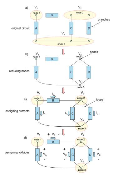
Fig. 3.1. An electric network and assigning branch voltages/currents.
