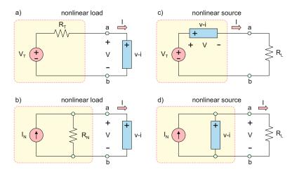
Fig. 4.20. Four basic nonlinear circuits.
