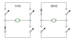
Fig. 13.15. Identification of two possible free run to a stop states. Two next states (1011 and 1000) are obtained by permutation.
