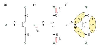
Fig. 17.2. Circuit symbol for the npn-junction transistor, terminal currents, and terminal voltages.
