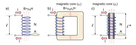
Fig. 6.11. Three types of a solenoid.
