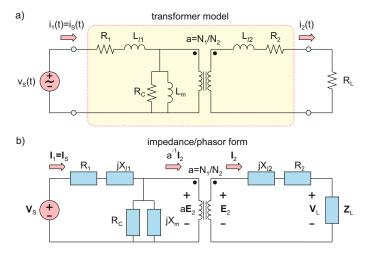
Fig. 12.17. Equivalent circuits for real transformers with harmonic source and linear load.
