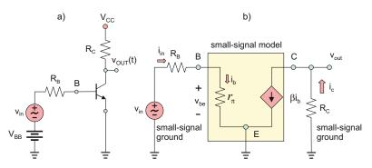
Fig. 17.36. Base-bias amplifier circuit and its small-signal model.
