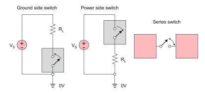
Fig. 13.2. Switch positions in a circuit.
