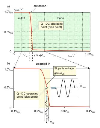
Fig. 18.28. Voltage transfer characteristic of the MOSFET common-source amplifier ( $\mathbf{a}$ ) and the amplification principle ( $\mathbf{b}$ ). The output sinusoidal signal indicates no distortion, which is a simplification. Circuit parameters are those from Exercise 18.14.
