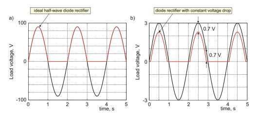
Fig. 16.21. Rectified (or load) voltage versus source voltage. (a) The result for the ideal half-wave diode rectifier or rectifier with a high input signal. (b) The result using the constant-voltage-drop-diode model for a moderate input signal.
