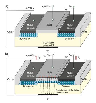
Fig. 13.5. Simplified diagram of transistor conduction for an n-channel MOSFET: (a) zero control voltage and (b) control voltage approaching the threshold value.
