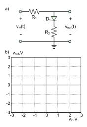
**Problem 16.77.** Repeat Problem 16.76 for the diode circuit shown in the figure below. Assume  $R_1 = 1 \text{ k}\Omega$ ,  $R_2 = 1 \text{ k}\Omega$ , and  $R_3 = 1 \text{ k}\Omega$ . Label the endpoint voltages.
