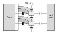
Fig. 12.18. Internal winding capacitances of a realistic high-frequency transformer.
