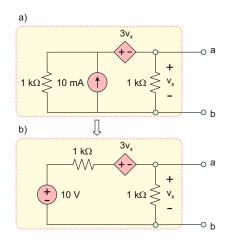
Fig. 4.15. A network with dependent sources to be converted to its equivalent forms.
