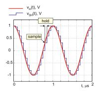
Fig. 14.22. Analog continuous voltage versus sample-and-hold voltage.
