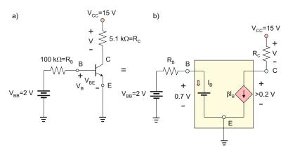
Fig. 17.16. Transistor circuit solved using the method of assumed states.
