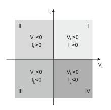
Fig. 13.8. Quadrants of load voltage and load current.
