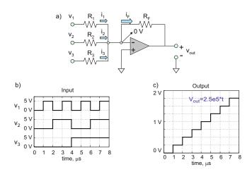
Fig. 5.15. (a) Circuit diagram of a summing amplifier. (b) and (c) Typical input and output voltages.
