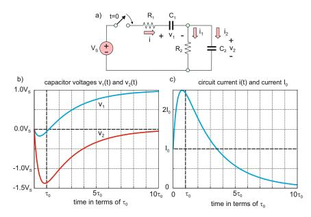
Fig. 7.25. A non-STC circuit with two resistances and two capacitances and its solution behavior.
