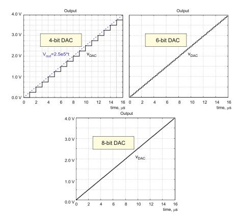
Fig. 14.17. Comparative resolution of the 4-bit DAC, the 6-bit DAC, and the 8-bit DAC. In all three cases, the full-scale output voltage range (4 V) is the same. The linear time dependence,  $v_{out}(t) = 2.5 \times 10^5 t$  (V), over the time interval from 0 to 16 µs is approximated.
