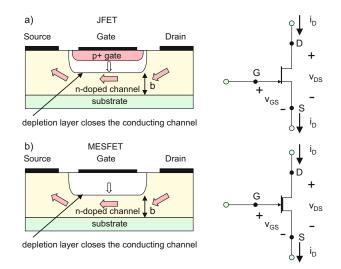
Fig. 18.10. Two schematic FET configurations: (a) n-channel JFET and (b) n-channel MESFET. A variant for both configurations is the dual gate arrangement. You should note that the corresponding circuit symbols have a continuous gate, denoting the normally "on" state.
