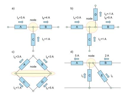
Fig. 3.2. Different types of the nodes in an electric network subject to KCL.
