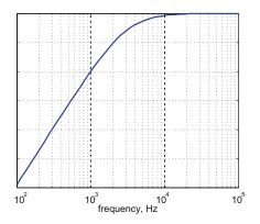
**Problem 9.25.** Prove analytically that the amplitude transfer functions of the low-pass filter and the high-pass filter are the mirror reflections of each other about the break frequency in the Bode plot.
