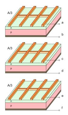
**Problem 4.23.** Individual solar cells in the figure to the previous problem are to be connected into a standard solar module. Draw the corresponding wire connections.
