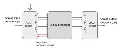
Fig. 14.25. DSP block diagram. The ADC converter still needs to be completed.
