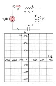
**Problem 10.8.** In the series resonant RLC circuit shown in the figure below, given  $V_m = 5 \text{ V}$ ,  $L = 30 \text{ }\mu\text{H}$ , C = 0.48 nF,  $R = 50 \Omega$ :
