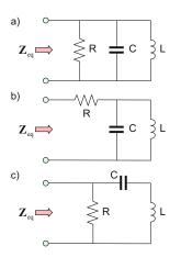
**Problem 8.53.** A complex impedance of any circuit may be written in the form  $\mathbf{Z} = R + jX$  where *R* is called the resistance and *X* is called the *electrical reactance* or simply the *reactance*. An engineer measures a reactance of 2  $\Omega$  over an inductor at 60 Hz. What is the inductance?
