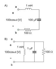
**Problem 11.21.** Determine the average power delivered to the load circuit shown in the figure below. The AC signal frequency is  $10^6$  Hz.
