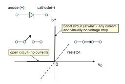
Fig. 16.9. The v-i characteristics of an ideal diode. The resistor v-i characteristic is a dashed line.
