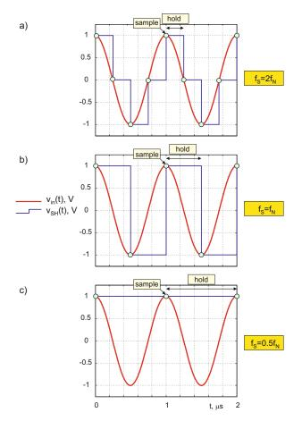
Fig. 14.24. Effect of sampling rate on the sample-and hold voltage.
