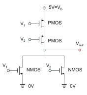
Fig. 13.21. CMOS NOR logic gate.
