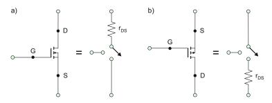
Fig. 18.19. MOSFET resistor-switch model in the triode region.
