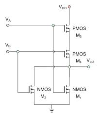
**Problem 18.38.** For a logic gate shown in the figure that follows, construct the truth table in the form of Table 18.7 and determine the output gate resistance for *every* input voltage combination. Assume  $V_{\text{DD}} > V_{\text{Th}}$  for the NMOS transistor and  $V_{\text{DD}} > |V_{\text{Th}}|$  for the PMOS transistor. Label turn-on resistances of  $M_{1,2,3,4,5,6}$  as  $r_{\text{DS}1,2,3,4,5,6}$ .
