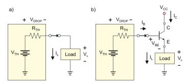
Fig. 17.26. Voltage divider circuit comparison after applying their Thévenin equivalents.
