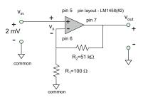
**Problem 5.26.** Determine the output voltage of the ideal operational amplifier shown in the figure. The amplifier is driven by a  $\pm 10$ -V dual power supply.
