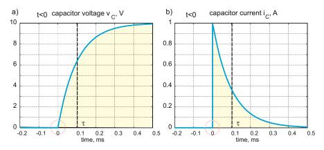
Fig. 7.8. Voltage/current plots for charging a  $10-\mu$ F capacitor in series with a  $10-\Omega$  resistor. We again observe continuity of the capacitor voltage (the "capacitor inertia").
