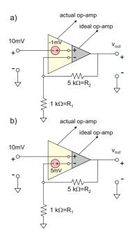
**Problem 5.63.** Determine the output voltage to nonideal operational amplifier circuits (with nonzero input currents) shown in the figures below. The input terminal is connected directly to the common terminal (grounded). The strength of every bias current source is 100 nA. *Hint:* The upper bias current source does not contribute to the solution.
