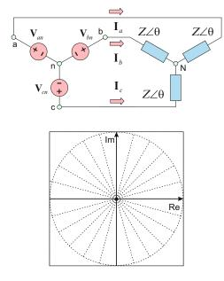
**Problem 11.44.** In the balanced three-phase wye-wye circuit shown in the figure that follows, the power line resistance and inductance are additionally included into consideration. The three-phase source operates at 60 Hz;  $R = 2 \Omega$ , L = 9.6 mH. You are given the *abc* sequence of phase voltages  $V_{an} = 170 \angle 0^{\circ}$  [V],  $V_{bn} = 170 \angle -120^{\circ}$  [V],  $V_{bn} = 170 \angle 120^{\circ}$  [V], and load impedance per phase,  $\mathbf{Z} = 7 + j30 \Omega$ .
