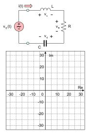
**Problem 10.9.** A series resonant LC circuit is driven by a laboratory AC voltage source with an amplitude  $V_{\rm m} = 12$  V and an internal resistance of 50  $\Omega$  (a function generator). Which value should the ratio L/C have to obtain the amplitude of the capacitor voltage equal to 200 V at the resonance?
