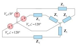
**Problem 11.41.** Prove that Eq. (11.28) of this chapter for line voltages also holds for the negative phase sequence to within the substitution  $30^{\circ} \rightarrow -30^{\circ}$ .
