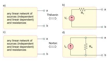
Fig. 4.11. Thévenin's and Norton's theorems: replacing linear active circuits by its Thévenin and Norton equivalents.
