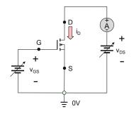
**Problem 18.31.** For the circuit shown in the figure that follows, determine the region of MOSFET operation as well as the drain current  $i_D$  for each set of conditions given. Assume  $k_p = 100 \text{ mA/V}^2$  and  $V_{\text{Th}} = -2 \text{ V}$ .
