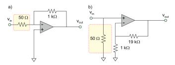
Fig. 5.22. Two possible amplifier configurations matched to a 50- $\Omega$  input resistance.
