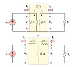
Fig. 12.22. Conversion of two coupled inductors to the T-network of three inductances.
