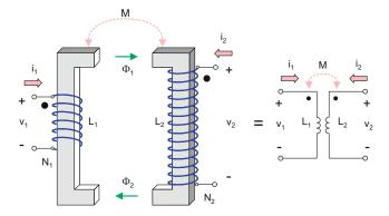
Fig. 12.19. Two coupled inductors. Note that we no longer use the transformer symbol. Also note the passive reference configuration for each inductance.
