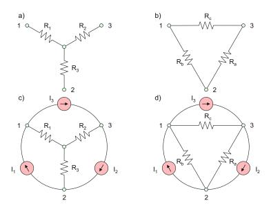
Fig. 3.27. (a) Y (wye) and (b)  $\Delta$  (delta) networks; (c) and (d) applying the superposition theorem to establish network equivalence.
