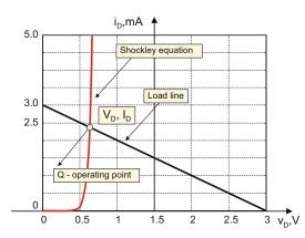
Fig. 16.15. Shockley's equation to scale and the load line for the circuit in Fig. 16.14.
