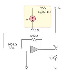
**Problem 5.58.** An amplifier circuit is needed with the closed-loop gain  $A_{\rm CL} = +1000$ . The input resistance (impedance) to the circuit should be 5 k $\Omega$ . Present two alternative circuit diagrams and specify the necessary resistor values. The first circuit must use inverting amplifiers and the second circuit-non-inverting amplifiers.
