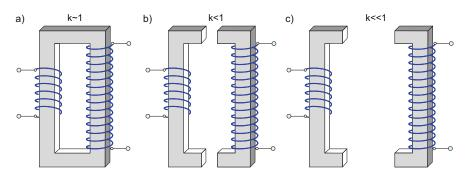
Fig. 12.23. Different configurations and coupling coefficient values for two coupled inductors.
