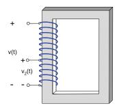
**Problem 12.4.** For the circuit shown in the figure below, determine voltage  $v_2(t)$  if  $v(t) = 70 \cos \omega t$  [V] using Faraday's law of induction. Count the number of turns. Assume no flux leakage.
