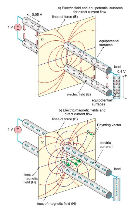
Fig. 1.7. Accurate physical model of an electric circuit.
