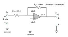
**Problem 5.29.** Determine the output voltage of the ideal operational amplifier shown in the figure. The amplifier is driven by a  $\pm 10$ -V dual power supply.
