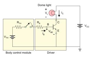
Fig. 17.30. Automotive dome light application.
