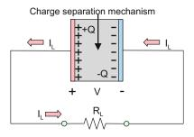
Fig. 2.26. Power source schematically represented as a capacitor continuously charged by a charge separation mechanism—the *charge pump*.
