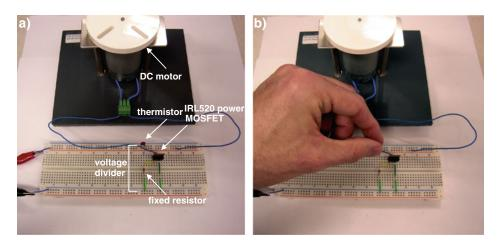
Fig. 3.20. Laboratory realization of the circuit shown in Fig. 3.19.
