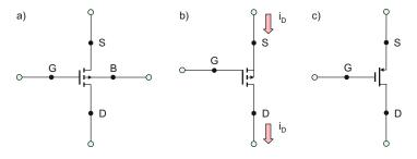
Fig. 18.8. Circuit symbols of (a) a four-terminal PMOS transistor, (b) a three-terminal asymmetric PMOS transistor with the body tied to the source, and (c) the same but simplified symbol.
