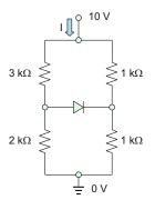
**Problem 16.24.** For the circuit below find circuit current *I*, assuming that both diodes are ideal. The ground path is simultaneously the current return path.
