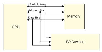
Fig. 15.1. Architecture of a generic computer.
