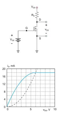
**Problem 18.40.** In a fixed-gate NMOS transistor circuit shown in the figure that follows, the NMOS transistor has the lumped process parameter  $k_n = 1.0 \text{ mA/V}^2$  and the threshold voltage of 1.0 V. Furthermore,  $V_{\text{DD}} = 15 \text{ V}$ , and  $R_{\text{D}} = 1 \text{ k}\Omega$ . Determine the region of operation of the transistor and find the solution for the drain-source voltage  $v_{\text{DS}}$  and drain current  $i_{\text{D}}$  when
