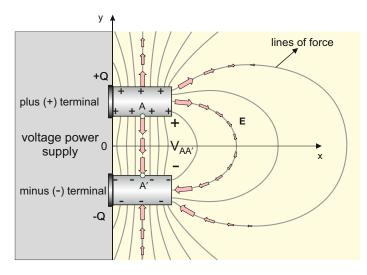
Fig. 1.1. Electric field emanating from a voltage supply with open-circuit output terminals.
