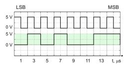
Fig. 14.9. Timing diagram for a binary bit steam.
