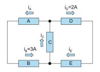
**Problem 3.7.** Find a relation between currents  $i_{\rm C}$ ,  $i_{\rm E}$  for the circuit shown in the following figure. Does the problem have a unique solution?
