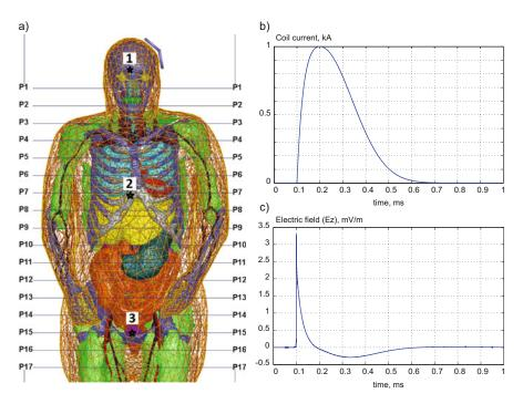
Fig. 9.18. Time-domain computational solution for the induced electric field within a human body obtained from the frequency-domain data via the FFT.
