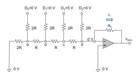
**Problem 14.39.** An important step in the analysis of the R/2R ladder network is finding Thévenin equivalent for the circuit shown in the figure. Find the Thévenin equivalent and draw the corresponding circuit.
