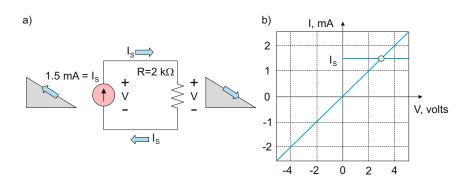
Fig. 2.24. Electric circuit solution in the graphical form.
