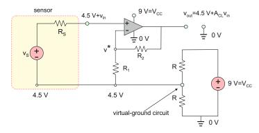
Fig. 5.27. A non-inverting amplifier driven by a single voltage supply, a battery. Absolute voltages versus ground (negative terminal of the battery) are shown.
