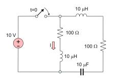
**Problem 6.38.** Find current *I* in the circuit shown in the figure at  $t \to \infty$ , in the DC steady state. The switch closes at t = 0.
