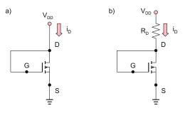
Fig. 18.24. Diode-connected MOSFET circuit with  $v_{GS} = v_{DS}$ .
