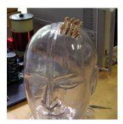
Fig. 12.21. An array of coupled inductors (small coils) located on top of a human-head phantom. This hypothetic setup was tested for applications related to brain stimulation.
