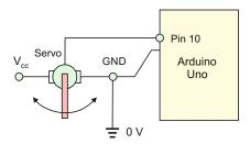
Fig. 15.16. Attaching a servomotor to the Arduino Uno.
