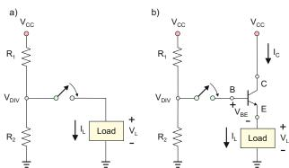
Fig. 17.25. Voltage divider circuit comparison.
