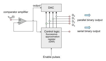
Fig. 14.27. A 4-bit successive-approximation ADC. Note that both parallel and serial outputs are allowed.
