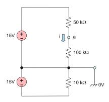
**Problem 3.68.** Determine the absolute voltage (versus chassis ground) and the current *i* at the circuit point *a*.
