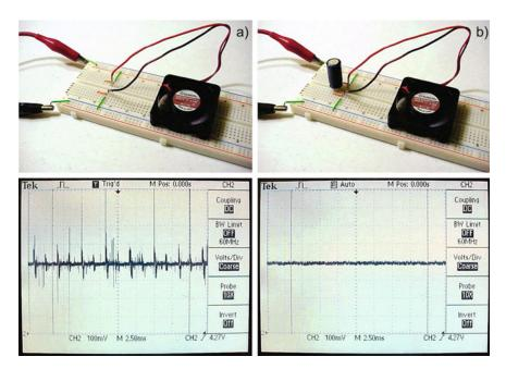
Fig. 6.20. Effect of bypass capacitor on the high-frequency noise created by a DC motor.
