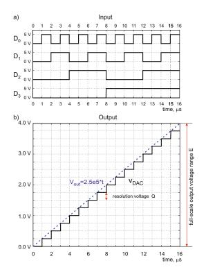
Fig. 14.16. Input digital voltages (a *4-bit binary counter*) and output analog voltage to the 4-bit digital-to-analog converter.
