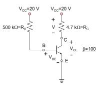
**Problem 17.31.** For three-transistor circuit shown in the figure, find the collector current  $I_{\rm C}$  and collector-to-emitter voltage  $V_{\rm CE}$
