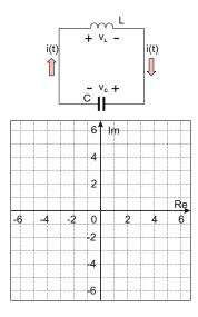
**Problem 10.3.** For a series ideal LC circuit shown in the figure below, the voltage source has the form  $v_{\rm S}(t) = V_{\rm m} \cos \omega t$ . Given  $V_{\rm m} = 5$  V, L = 0.5 mH, C = 1 µF:
