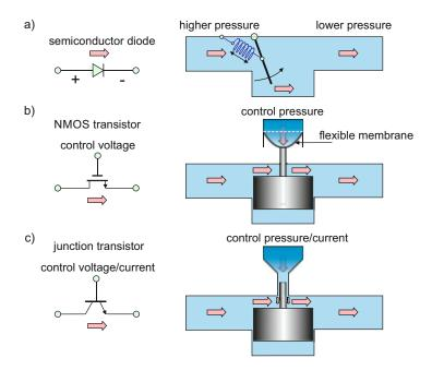
Fig. 1.11. Analogies for semiconductor circuit components.
