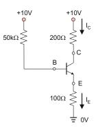
**Problem 17.37.** For the circuit shown in the figure, determine the transistor current gain  $\beta$ . Use the large-signal DC circuit model of the transistor.
