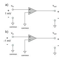
**Problem 5.33.** Each of the circuits shown in the figures below employs negative feedback. Find the output voltage  $v_{out}$  vs. ground (or common). *Hint:* The ground symbol in an amplifier circuit usually has the *same* meaning as the common port.
