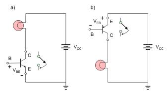
Fig. 17.27. Negative-side and positive-side BJT switches.
