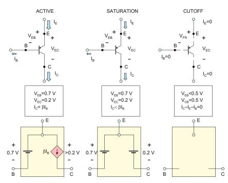
Fig. 17.15. Large-signal DC circuit model of a pnp BJT transistor.
