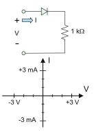
**Problem 16.28.** Sketch *I* versus *V* to scale for the circuit shown in the figure. Assume the ideal-diode model and allow *V* to range from -5 V to 5 V.
