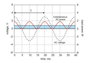
Fig. 11.1. Power (*solid line*) for a load voltage  $v(t) = 3 \cos(2\pi 50t)$  [V] (*dotted line*).
