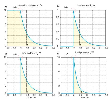
Fig. 7.2. (a) Capacitor voltage, (b) load current (c) load voltage, and (d) load power for a  $10-\mu$ F capacitor discharging into a  $10-\Omega$  load resistor.
