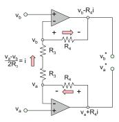
Fig. 5.33. Next step toward the instrumentation amplifier: we convert the non-inverting stage to a unity common-mode gain amplifier.
