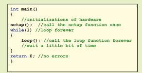
Fig. 15.10. The translation of the basic Arduino program code to C code.
