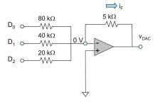
**Problem 14.26.** For a 4-bit binary-weightedinput DAC, the input voltages  $D_3, D_2, D_1, D_0$ are either 0 V or 5 V. The resolution voltage Q of 10 mV is required:
