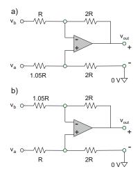
**Problem 5.84.** For the difference-amplifier circuit shown in the figure below, find the *differential-mode resistance (impedance)* to the amplifier. The differential-mode resistance is defined as the ratio of a voltage of a power supply placed between terminals a and b to the current that flows through this power supply.
