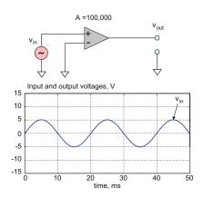
**Problem 5.13.** In a circuit shown in the figure below, an operational amplifier is driven by a  $\pm 15$ -V dual power supply (not shown). The open-circuit gain of the amplifier is A = 100,000. Sketch to scale the output voltage to the amplifier when
