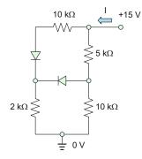
**Problem 16.25.** For the circuit shown in the figure below, find circuit current *I*, assuming that the diodes are ideal. The ground path is simultaneously the current return path.
