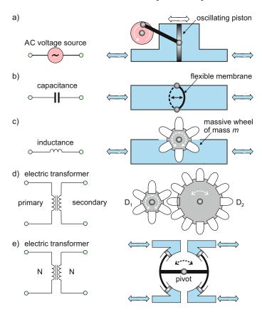
Fig. 1.10. Hydraulic analogies for alternating-current (AC) circuit elements.
