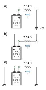
**Problem 2.54.** What is the voltmeters' (ammeter's) reading in the figure below?
