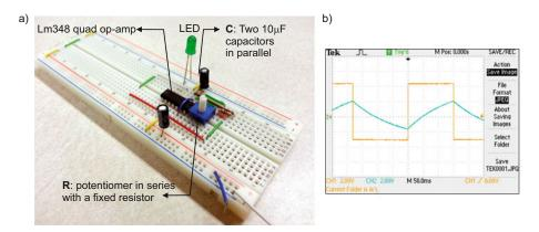
Fig. 7.22. (a) Timer circuit operation in laboratory. The square waveform is the output voltage  $v_{out}(t)$ . The curved waveform is the capacitor voltage  $v_C(t)$ . A variable resistance *R* makes it possible to visually control the oscillation frequency using an LED connected to the output through a *buffer amplifier*. The oscillation frequency changes from 0.5 to about 100 Hz.
