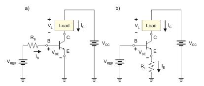
Fig. 17.23. Simple BJT configuration as constant-current sources.
