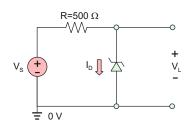
**Problem 16.52.** In a typical 12-V automotive application, battery voltage may vary between 10.5 and 14.1 V. The ECM (engine control module) determines fuel delivery and spark advance to control emissions based on several sensors connected to the engine. Many of these sensors require a stable 5-V reference that can be achieved through the use of a Zener diode. The figure that follows shows
