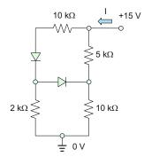
**Problem 16.26.** The circuit shown in the figure below can be used as a signaling system using one wire plus a common ground return. At any moment, the input has one of three voltage values shown in the figure. What is the status of the lamps for each input value?
