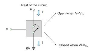
Fig. 2.15. Three-terminal unidirectional threshold switch (pull-down switch).
