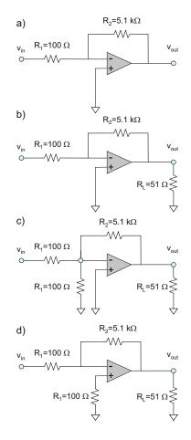
**Problem 5.36.** An inverting amplifier that achieves high-gain magnitude with a smaller range of resistance values is shown in the figure below. Find its output voltage  $v_{out}$  vs. ground (or common port) and the resulting amplifier gain.
