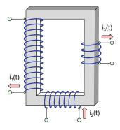
**Problem 12.9.** For the circuit shown in the figure below, determine current  $i_2(t)$  given that  $i_1(t) = 1 \cos \omega t$  [A]. Count the number of turns.
