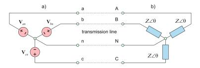
Fig. 11.16. Wye configuration for the three-phase source connected to a three-phase load.
