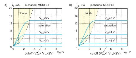
Fig. 18.14. (a) Drain current as a function of the drain-source voltage for an NMOS transistor with  $V_{\rm Th} = 2$  V and  $k_n = 3$  mA/V<sup>2</sup>. (b) Drain current as a function of the source-drain voltage for a PMOS transistor with  $|V_{\rm Th}| = 2$  V and  $k_p = 3$  mA/V<sup>2</sup>.
