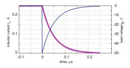
**Problem 7.38.** A 2-mH inductor, shown in the following figure, releases its energy into two  $1-k\Omega$  load resistors. The supply current is 100 mA.
