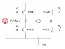
**Problem 13.23.** In the H-bridge circuit shown in the figure to the previous problem, the control voltages  $V_1$ ,  $V_2$ ,  $V_3$ ,  $V_4$  are either 0 V or 12 V. If we denote the 0-V control voltage by digit 0 (low) and the 12-V control voltage by digit 1 (high), all possible combinations of the control voltages are covered by the table that follows (the table in fact lists all *binary numbers* from 0 to 15). Fill out the table using five states:
