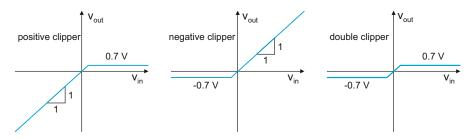
Fig. 16.35. Transfer characteristics of diode clipper circuits.
