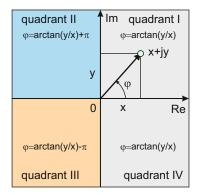
Fig. 8.5. A phasor in rectangular, or polar, form in the complex plane and the corresponding phase conversion. The phase of the complex number  $\varphi$  is given for different quadrants.
