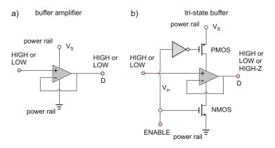
Fig. 14.12. Concept of a tri-state buffer.
