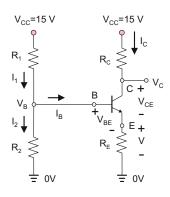
Fig. 17.20. Four-resistor bias circuit.
