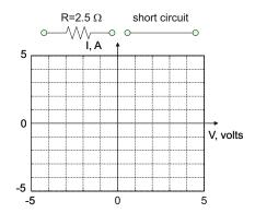
**Problem 2.4.** Given *v*-*i* characteristics of a resistance determine the corresponding conductance. Show units.
