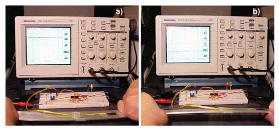
Fig. 5.35. Operation of the instrumentation amplifier with the strain gauge attached to a metal slab. (a) A "positive" bending moment is applied and (b) a "negative" bending moment is applied. The oscilloscope resolution is 1 V per division in every case.
