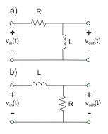
**Problem 9.34.** For the filter circuit shown in the figure below, assume the values  $R_1 = 628$   $\Omega$  and  $L_1 = 10$  mH.
