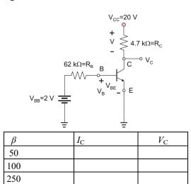
**Problem 17.35.** For the circuit shown in the figure, fill the table that follows. Use the large-signal DC circuit model of the transistor.
