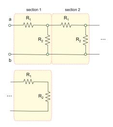
*Hint:* For the semi-infinite ladder network in the previous figure, the equivalent resistance  $R_{eq}$  will not change after adding a new section up front as shown in the figure that follows:
