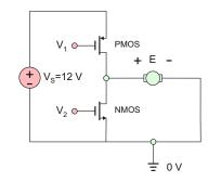
**Problem 13.20.** In the half H-bridge circuit shown in the figure to the previous problem, the control voltages  $V_1$ ,  $V_2$  are either 0 V or 12 V. If we denote the 0-V control voltage by 0 (low) and the 12-V control voltage by 1 (high), all possible combinations of the control voltages are covered by the table that follows (the table in fact lists all *binary numbers* from 0 to 3). Fill out the table using four states:
