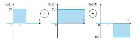
Fig. 7.33. A one-bit excitation voltage constructed as the sum of two step responses.
