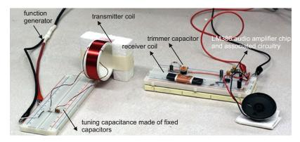
Fig. 10.21. Prototype of the near-field link implemented in laboratory.
