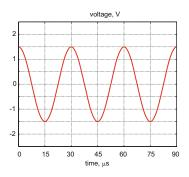
**Problem 14.41.** Determine frequency in Hz, angular frequency in rad/s, and amplitude of the harmonic voltage signal shown in the following figure.
