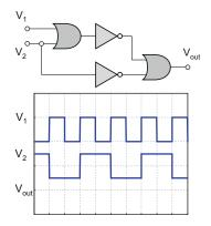
**Problem 13.58.** Given the logic circuit and the input waveforms in the following figure, draw the output waveform on the same figure. *Hint:* Construct the truth table of the logic circuit first.
