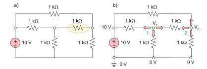
Fig. 4.2. Major steps of the nodal analysis applied to a circuit with a voltage source.
