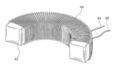
Fig. 10.24. A half-toroidal (*horseshoe*) coil used to concentrate the magnetic field between its tips in a molten metal detector (Foley, Biederman, Ludwig, and Makarov, US Patent 7,828,043 Nov. 9th 2010).
