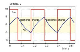
Fig. 7.21. Relaxation oscillator operation for the idealized amplifier model (amplifier hits the rails in saturation); the amplifier supply voltage is 10 V.
