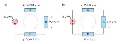
Fig. 3.4. KVL applied to a closed loop with one voltage source and three passive circuit elements. The dotted arrow indicates current flow in clockwise direction.
