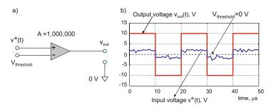
Fig. 5.3. A simple operational amplifier as a voltage comparator.
