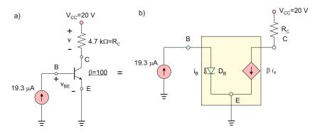
Fig. 17.12. A base-bias transistor circuit and its equivalent representation.
