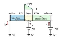
Fig. 17.5. Transistor test circuit of the common-emitter configuration in the active region.
