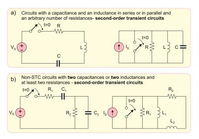
Fig. 7.29. Classification of second-order transient circuits.
