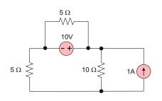
**Problem 3.70.** Determine the unknown current *I* in the circuit (solve by superposition).
