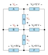
**Problem 3.15.** Determine voltage  $V_{\rm E}$  for the circuit shown in the following figure.
