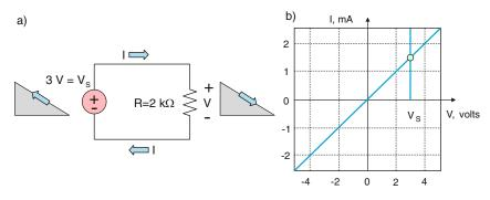
Fig. 2.19. Electric circuit solution in graphical form.
