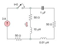
**Problem 6.41.** Find the voltage across the capacitance in the DC steady state and label its polarity in the figure at  $t \to \infty$ , in the DC steady state. The switch opens at t = 0.
