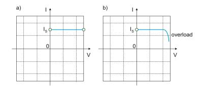
Fig. 2.22. v-i Characteristics of (a) an ideal current source and (b) its physical counterpart.
