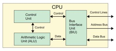
Fig. 15.2. Block diagram of a CPU.
