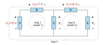
Fig. 3.5. KVL applied to a network with three loops, two meshes, and five circuit elements.
