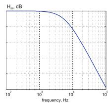
**Problem 9.24.** An amplitude Bode plot for a certain RC filter is shown in the figure below.
