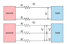
Fig. 11.25. Comparison of single-phase and three-phase transmission systems.
