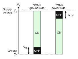
Fig. 13.4. Switching diagram for two MOSFET transistors.
