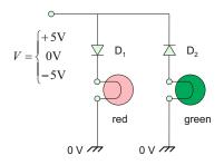
**Problem 16.27.** Sketch *I* versus *V* to scale for the circuit shown in the following figure. Assume the ideal-diode model and allow *V* to range from -3 V to 3 V.
