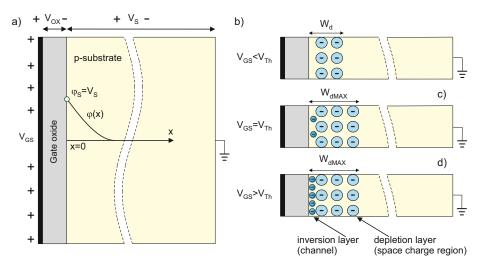
Fig. 18.5. (a) Central region of the MOSFET under an applied voltage  $v_{GS}$ : the MOS capacitor. (b) to (d) Formation of the depletion and inversion layers in the substrate. The entire region close to the semiconductor surface is called the *surface space-charge region*.
