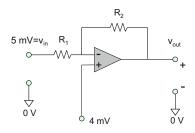
**Problem 5.67.** In the previous problem, denote the terminal voltage of 4 mV by  $V_{\text{off}}$ , the input voltage of 5 mV by  $v_{\text{in}}$ , the output voltage by  $v_{\text{out}}$ , and the amplifier gain by  $A_{\text{CL}}$ . Derive an analytical formula that determines  $V_{\text{off}}$  in terms of  $v_{\text{in}}$  given that the output voltage to the amplifier is exactly zero.
