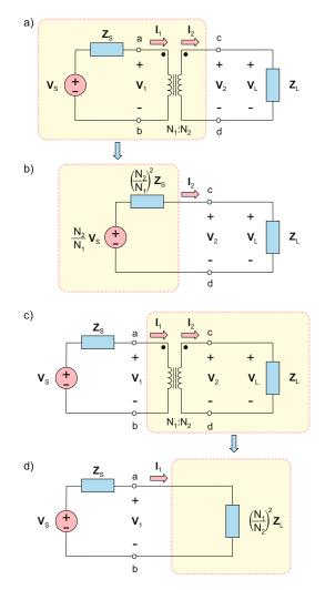
Fig. 12.6. (a) A source circuit and a load circuit connected to a transformer. (b) Equivalent circuit of the source with the transformer *when looking from the load*. (c) The same as (a). (d) Equivalent circuit of the load with the transformer *when looking from the source*.
