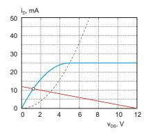
**Problem 18.42.** In the circuit shown in the figure that follows, the NMOS transistor has the lumped process parameter  $k_n$  and the threshold voltage  $V_{\text{Th}}$ . Derive the analytical expression for the drain current  $i_{\text{D}}$  as a function of  $V_{\text{DD}}$  valid for any values of  $V_{\text{DD}}$ .
