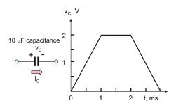
**Problem 6.31.** A 10- $\mu$ F capacitance is charged by the current  $i_{\rm C} = 1 \,\mathrm{mA} \cdot \cos^2(1000t)$ . At t = 0, the capacitance voltage is zero.
