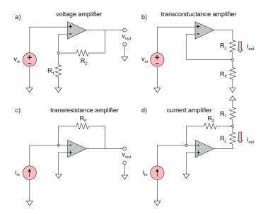
Fig. 5.38. Four basic amplifier types with negative feedback.
