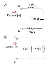
**Problem 11.20.** Determine the average power delivered to the load circuit between terminals a and b shown in the figure that follows. The AC angular frequency is 1000 rad/s.
