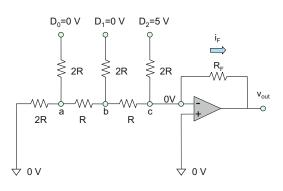
**Problem 5.46.** By solving the amplifier circuit shown in the following figure, determine its output voltage in terms of resistances  $R, R_F$ , given the input voltages  $D_0 = 0$  V,  $D_1 = 5$  V,  $D_2 = 0$  V.
