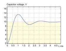
**Problem 7.101.** Capacitor voltage is measured in a series RLC circuit as shown in the figure to the previous problem. Given  $R = 2\Omega$ , estimate circuit inductance L and circuit capacitance C.
