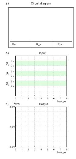
**Problem 14.30.** A 4-bit binary-weighted-input DAC has the resolution voltage, Q, of 0.125 V and the input voltages shown in the following figure. Pin  $D_3$  is accidentally connected to ground. Plot the output voltage of a DAC to scale versus time.
