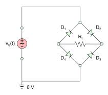
Fig. 16.24. The full-wave diode bridge rectifier: four diodes are bridged by the load resistor  $R_{\rm L}$ .
