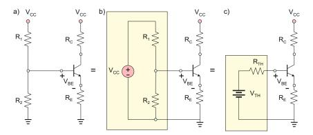
Fig. 17.21. Solution of the four-resistor bias circuit using the method of Thévenin equivalent.
