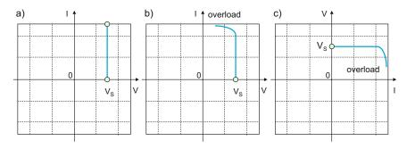
Fig. 2.17. v-i Characteristics for (a) ideal voltage source used in the circuit analysis and (b) its physical counterpart—a regulated laboratory power supply. (c) Typical way of drawing the v-i characteristic for the voltage source with the axes interchanged.
