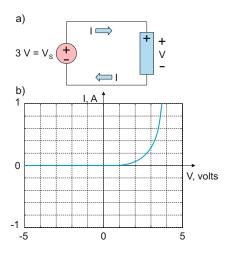
The polarity (direction of current inflow for passive reference configuration) of the element is labeled by a sign plus. The v-i characteristic of the element is also shown in the figure. Determine current I and voltage V.
