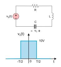
**Problem 7.84.** Repeat the previous problem for the voltage source shown in the figure that follows (a voltage pulse train of two bits).
