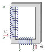
**Problem 12.8.** For the circuit shown in the following figure, establish the relation between currents  $i_1(t)$ ,  $i_2(t)$ , and  $i_3(t)$ . Assume an ideal magnetic core. Count the number of turns.
