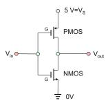
Fig. 13.19. CMOS logic inverter or NOT gate.
