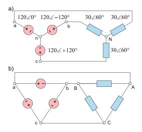
**Problem 11.53.** A three-phase balanced deltadelta system is shown in the figure that follows. Its wye-wye equivalent is sought, which is shown in the same figure. For the wye-wye system, write the corresponding voltage and impedance values in the phasor form close to every circuit element.
