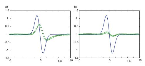
Fig. 9.17. *Diamonds*: HPF output for (**a**)  $\omega_0 = 1$  rad/s and (**b**)  $\omega_0 = 10$  rad/s, respectively. *Solid curve*: analytical derivative of the input Gaussian pulse.
