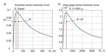
Fig. 3.18. Sensitivity curves for the divider sensor circuits with a thermistor and a strain gauge.
