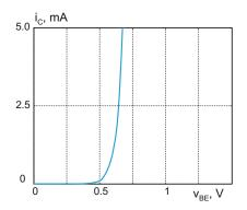
Fig. 17.7. Typical dependence of the collector current on  $v_{\rm BE}$ .
