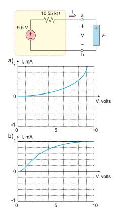
**Problem 4.65.** A circuit shown in the following figure contains a nonlinear passive element as part of a current source. Using the load line method, approximately determine the voltage across the element and the current through it for the *v*-*i* characteristic of the nonlinear element shown in the same figure.
