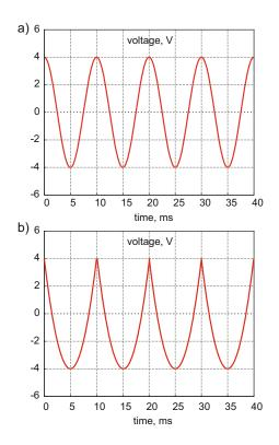
**Problem 11.13.** Of the two periodic signals shown in the figure that follows, which signal delivers more average power into a resistive load? The periodic voltage on the top graph is the cosine function. Explain your answer and provide:
