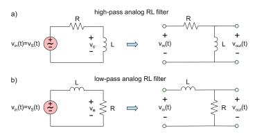
Fig. 9.9. (a) Transformation of a series RL circuit into a high-pass analog RL filter. (b) Similar transformation into the low-pass RL filter.
