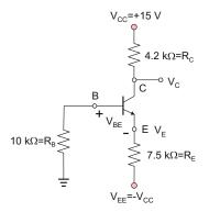
Fig. 17.22. A bias circuit with the dual-polarity power supply.
