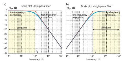
Fig. 9.5. (a) Bode plot for the amplitude transfer function of the low-pass RC filter with the break frequency  $f_b = 1$  kHz. (b) The same Bode plot but for the high-pass RC filter. Note high-frequency and low-frequency asymptotes.
