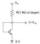
**Problem 13.12.** A circuit shown in the figure below is used to measure the threshold voltage of the PMOS transistor. Could you explain why? *Hint:* Determine all possible values of the voltage *V*.
