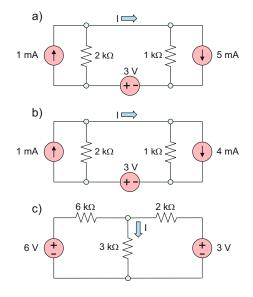
**Problem 4.45.** Solve the circuits shown in the following figure—determine unknown voltage *V* or current *I* (show units). You can use any of the methods studied in class:
