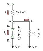
Fig. 16.18. Diode voltage reference for the load resistor  $R_{\rm L}$ .
