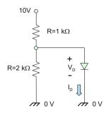
**Problem 16.21.** Assuming the ideal-diode model, find current I for the circuit shown in the figure below.
