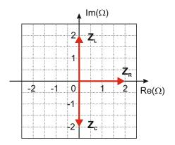
Fig. 8.12. Complex impedances displayed in the phasor diagram.
