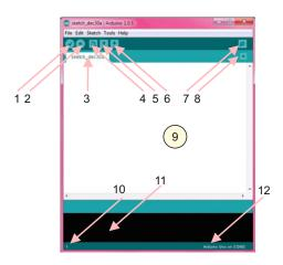
Fig. 15.8. The various parts of the Arduino IDE environment.
