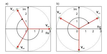
Fig. 11.15. (a) Phasor diagram for the phase sequence 0,  $+120^{\circ}$ ,  $-120^{\circ}$  and (b) phasor diagram for individual phase voltages from Eq. (11.42). Both three-phase sources are equivalent.
