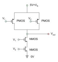
Fig. 13.25. CMOS NAND logic gate.
