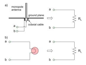
Fig. 2.11. (a) Radiating monopole antenna is modeled as a resistance. (b) Light source is approximately modeled as a resistance.
