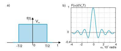
Fig. 9.14. (a) Rectangular pulse f(t) of duration  $T = 1 \mu s$  and (b) its Fourier spectrum in the form of a sinc function.
