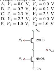
**Problem 13.7.** For the circuit shown in the figure below,  $V_{\rm S} = 2.5$  V and  $V_{\rm Tn} = 0.5$  V. Determine the output voltage  $V_{\rm out}$  when:
