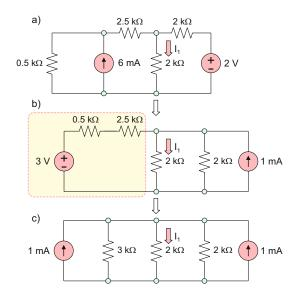
Fig. 4.9. Circuit modifications using the source transformation theorem.
