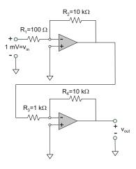
**Problem 5.56.** A sensor with Thévenin voltage (source voltage)  $v_{\rm S} = 2.5$  mV shown in the figure is to be connected to an amplifier circuit. An amplified replica of the sensor's voltage,  $v_{\rm out} \approx 1000 v_{\rm S}$ , is needed at the circuit's output.
