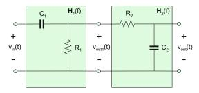
Fig. 9.7. Cascading a high-pass and a low-pass filter into a more complex filter structure.
