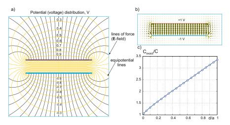
Fig. 6.4. (a) Equipotential lines and lines of force for a capacitor with d/a = 0.2 in the central cross-sectional plane (the plates are at  $\pm 1$  V). (b) Fringing electric field for the same capacitor observed in the central cross-sectional plane (the plates are at  $\pm 1$  V). (c) Ratio of the accurate capacitance values (found numerically) to the values predicted by Eq. (6.6).
