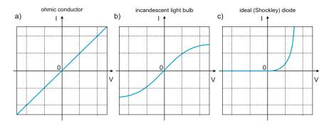
Fig. 2.12. Three *v*-*i* characteristics: (a) linear—resistance; (b) nonlinear—incandescent light bulb; and (c) nonlinear—ideal or Shockley diode.
