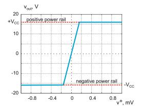
Fig. 5.2. Amplifier output voltage in the open-loop configuration. The open-loop gain is  $A_{OL} = 10^5$  and the supply voltage is  $\pm 16$  V. Note that the scale for the input voltage is in mV.
