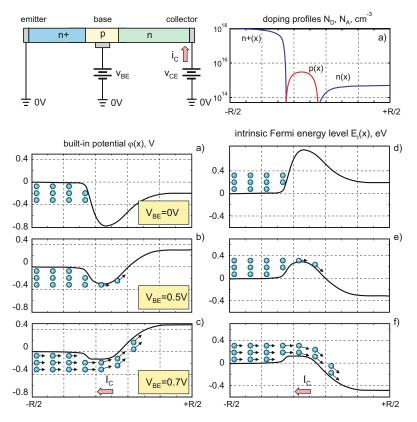
Fig. 17.3. Operation of the npn-junction transistor for three values of base-emitter voltage  $v_{\rm BE}$ . The collector-base voltage  $v_{\rm CB}$  is fixed at zero volts.
