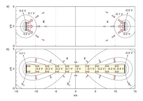
Fig. 1.6. (a) Two electrodes subject to  $\pm 0.5$  V in free space; (b) the same electrodes but with a conducting cylinder between them. Equipotential lines and electric field vectors are shown.
