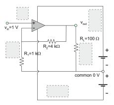
**Problem 5.42.** The amplifier shown in the figure below is powered by a  $\pm$ 9-V dual-polarity voltage power supply.
