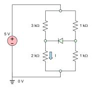
**Problem 16.22.** Assuming the ideal-diode model, find current I for the circuit shown in the figure below.
