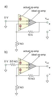
**Problem 5.64.** For the amplifier circuit shown in the figure below, determine the output voltage. Use  $R_1 = R_2 = 1 \text{ k}\Omega$ .
