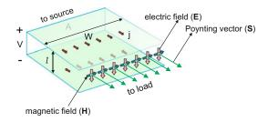
Fig. 1.8. Transmission line in the form of two current sheets.
