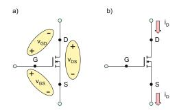
Fig. 18.3. Terminal voltages and currents for the NMOS transistor.
