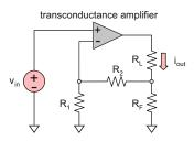
**Problem 5.101.** The amplifier circuit shown in the figure that follows is the *Howland current source* widely used in biomedical instrumentation; its output is the current through the load resistance.
