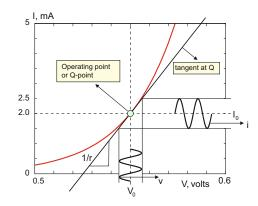
Fig. 2.13. Finding dynamic resistance for an ideal diode.
