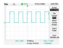
**Problem 14.7.** A Tektronix oscilloscope is measuring a voltage clock signal. The oscilloscope window is shown in the following figure.
