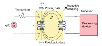
Fig. 10.16. The concept of the near-field wireless link; the magnetic flux density is shared between receiver and transmitter coils.
