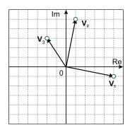
Fig. 8.8. Phasor diagram for three time-domain voltages  $v_1(t)$ ,  $v_2(t)$ ,  $v_3(t)$ . Voltage  $v_2(t)$  leads voltage  $v_1(t)$  by 90°, but lags voltage  $v_3(t)$ .
