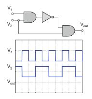
**Problem 13.59.** Given the logic circuit and the input waveforms in the following figure, draw the output waveform on the same figure. *Hint:* Construct the truth table of the logic circuit first.
