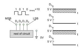
Fig. 14.3. Four parallel digital output voltages  $D_{3,2,1,0}$  of either 0 V or 5 V corresponding to a decimal number 10.
