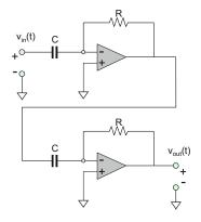
**Problem 6.49.** For the circuit shown in the following figure, express the output voltage,  $v_{out}(t)$ , as a function of time in terms of the input voltage,  $v_{in}(t)$ , and circuit parameters *R*, *C*. Assume ideal amplifiers.
