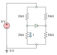
**Problem 16.23.** For the circuit shown in the figure below, determine circuit current I, assuming that the diode is ideal. The ground path is simultaneously the current return path.
