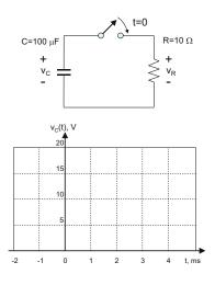
**Problem 7.7.** A 100- $\mu$ F capacitor, shown in the following figure, discharges into a 5- $\Omega$  load resistor. The capacitor is charged to 20 V prior to t = 0.
