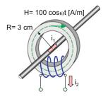
**Problem 12.10.** For the circuit shown in the figure below, establish the relation between currents  $i_1(t)$ ,  $i_2(t)$ , and  $i_3(t)$ . Assume an ideal magnetic core. Count the number of turns. *Hint*: Ampere's law for the ideal core applies to every closed path.
