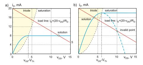
Fig. 18.23. Graphical representation of the solution for the DC circuit in Fig. 18.22 and intersection of the load line with the  $v_{DS}$ — $i_D$  curve. (a) NMOS transistor in saturation and (b) NMOS transistor in triode region.
