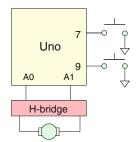
The circuitry should use two push button switches to choose the direction.
