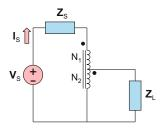
**Problem 12.36.** Find the equivalent input impedance,  $Z_{in}$ , for two autotransformer circuits shown in the following figure.
