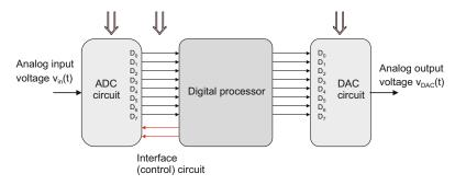
Fig. 14.1. Structure of a DSP including different circuit blocks.
