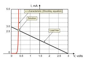
Fig. 4.22. Load line method applied to a nonlinear circuit with an ideal diode.
