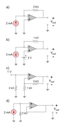
**Problem 5.34.** Each of the circuits shown in the figures below employs negative feedback. Find the output voltage  $V_{out}$  vs. ground (or common). *Hint:* The ground symbol in the amplifier circuit usually has the same meaning as the common port.
