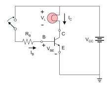
**Problem 17.49.** For the circuit shown in the figure below,  $V_{\rm CC} = 12$  V, and the bulb turn on resistance is 40  $\Omega$ . Assume the minimum value  $\beta = 30$ .
