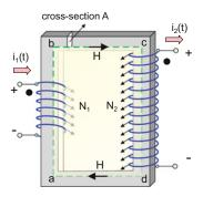
Fig. 12.2. Ampere's law for a transformer.
