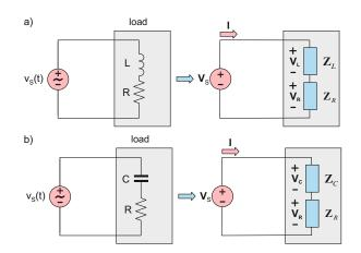
Fig. 11.7. Two circuits for power calculation of (a) inductive load and (b) capacitive load.
