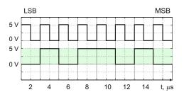
**Problem 14.9.** The following figure shows a timing diagram: the clock signal and the actual synchronized serial bit stream (the polar NRZ code).
