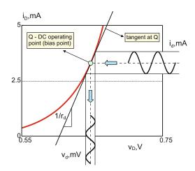
Fig. 16.16. Linearization procedure for a switching diode with n = 1.7,  $I_{\rm S} = 1.1$  nA at 25 °C.
