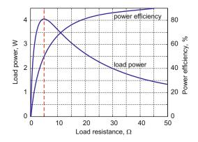
Fig. 4.19. Load power and power efficiency for fixed  $V_T = 9V$ ,  $R_T = 5\Omega$ .
