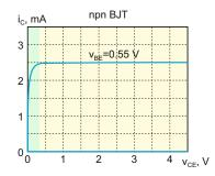
**Problem 17.12.** Using the Ebers-Moll transistor model, express the collector current  $i_{\rm C}$  in terms of the base current  $i_{\rm B}$  when the voltage across the transistor is exactly zero, i.e., when  $v_{\rm CE} = 0$ .
