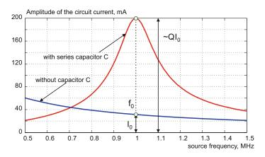
Fig. 10.18. Amplitudes of the circuit current for the original and modified circuits in Fig. 10.17.
