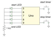
**Problem 15.56.** Write a program that turns the Arduino into a rudimentary stopwatch. The Arduino should begin "timing" after the push of a push button and then "stop" timing after a push of a different button. A sketch is shown in the following figure. *Hint:* Use some of the built-in timing features.
