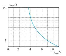
**Problem 18.36.** The datasheet for an IRF510 enhanced-mode n-channel power MOSFET from Fairchild reports the average drain-source on-state resistance  $r_{\rm DS} = v_{\rm DS}/i_{\rm D} = 0.4 \ \Omega$  for  $i_{\rm D} = 3.4 \text{ A}$  and  $v_{\rm GS} = 10 \text{ V}$ . Assuming threshold voltage to be 2.0 V, sketch  $r_{\rm DS}$  as a function of  $v_{\rm GS}$  to scale.
