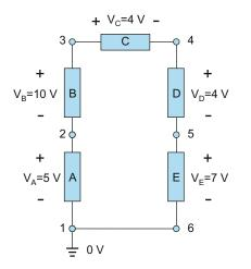
**Problem 2.58.** Determine voltages across circuit elements A, B, C, D, and E in the circuit shown in the following figure.
