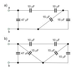
**Problem 6.12.** Find the equivalent capacitance for each circuit shown in the following figure.
