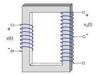
**Problem 12.5.** Explain the meaning of the ideal magnetic core. What is the inductance value for an inductor which uses the closed-loop ideal magnetic core?
