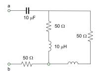
**Problem 6.43.** Determine the equivalent resistance between terminals a and b for the circuit shown in the following figure in the DC steady state.
