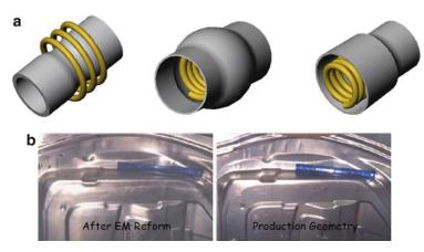
Fig. 7.5. (a) Electromagnetic forming of metal joints. The current in the windings generates a magnetic flux that induces eddy currents in the metal. Their product is the Lorentz force. (b) Electromagnetically reformed door panel compared with the production geometry.
