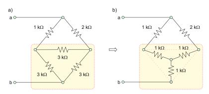
Fig. 3.28. Network simplification using  $\Delta$  to Y transformations.
