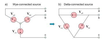
Fig. 11.28. Wye-connected source versus delta-connected source.
