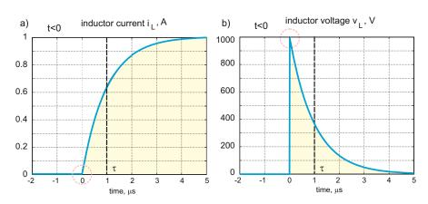
Fig. 7.13. Voltage/current plots for "charging" the 1-mH inductor in parallel with the 1-k $\Omega$  resistor.
