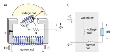
Fig. 11.9. (a) Wattmeter concept and (b) wattmeter coil connection to the load.
