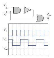
**Problem 13.57.** Given the logic circuit and the input waveforms in the following figure, draw the output waveform on the same figure. *Hint:* Construct the truth table of the logic circuit first.
