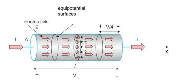
Fig. 2.5. Finding the resistance of a conducting cylinder.
