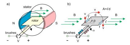
Fig. 2.27. Charge separation in a DC electromechanical generator.
