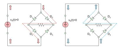
Fig. 16.25. Current flow in the full-wave diode bridge rectifier assuming ideal diodes. Circuit on the left is for positive applied voltage; circuit on the right is for negative applied voltage.
