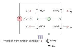
Fig. 13.17. Realization of the PWM with one more switching transistor added to the H-bridge. The control signal to the transistor gate is supplied by a function generator.
