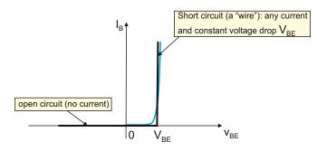
Fig. 17.13. Large-signal DC circuit model of the EBJ.
