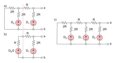
Fig. 4.14. Two-bit and three-bit *R*-2*R* ladder networks.
