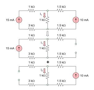
Fig. 3.26. Application of the superposition principle to current sources.
