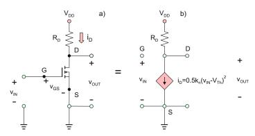
Fig. 18.27. MOSFET common-source amplifier model.
