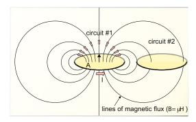
Fig. 6.10. Magnetic flux density generated by circuit #1.
