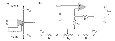
Fig. 5.25. (a) Output DC offset voltage for the LM741 is reduced to zero by adjusting the potentiometer placed between its offset-null pins and (b) a similar operation performed with the virtual ground of the feedback loop.
