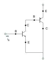
**Problem 17.17.** Repeat the previous problem if  $v_{\text{BE}}$  of the pnp transistor is 0.7 V.
