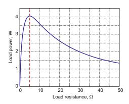
Fig. 4.18. Load power as a function of the load resistance for fixed  $V_T = 9$  V,  $R_T = 5 \Omega$ .
