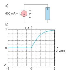
**Problem 2.36.** Plot to scale the *v*-*i* characteristic of the practical current source shown in the following figure.
