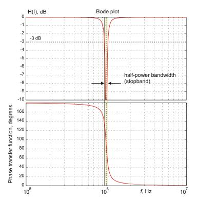
Fig. 10.14. Amplitude and phase Bode plots for the band-reject series RLC filter.
