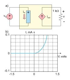
A nonlinear passive circuit element is shown by a rectangle. Element's polarity (direction of current inflow for passive reference configuration) of the element is labeled by a sign plus. The *v-i* characteristic of the element is also shown in the figure. The independent voltage source is given by  $v_{\rm S} = 0.6$  V; the short-circuit current gain of the dependent source is 100 A/A.
