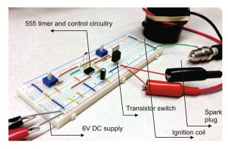
Fig. 7.16. A constructed ignition system.
