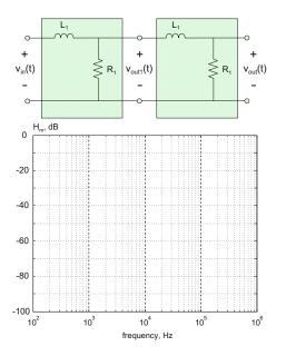
**Problem 9.35.** The transfer function of a filter circuit is given by  $H(f) = \frac{1+j(f/1000)}{1+(f/1000)^2}$ . Create its amplitude and phase Bode plots in the frequency band from 10 Hz to 100 kHz by finding transfer function values for (at least) every decade.
