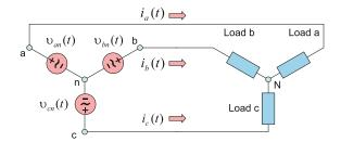
Fig. 11.24. Three-phase balanced wye-wye circuit in the time domain. Three individual loads are identical. Each of them is characterized by the impedance  $\mathbf{Z} = Z \angle \theta$  in the frequency domain.
