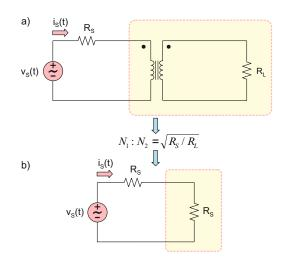
Fig. 12.7. (a) A matching transformer for real impedances. (b) Equivalent circuit of the load with the transformer *when looking from the source*.
