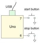
**Problem 15.57.** Implement a "lap" feature which spits out the time elapsed instead of stopping the count. A sketch is shown in the following figure.
