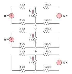
Fig. 3.25. Application of the superposition principle to voltage sources.
