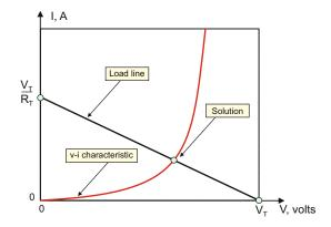
Fig. 4.21. Load line method for a nonlinear circuit.
