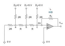
**Problem 14.38.** By solving the amplifier circuit, determine the output voltage of the 4-bit R/2R ladder DAC in Fig. 14.18 given that  $D_3 = 0$  V,  $D_2 = 5$  V,  $D_1 = 0$  V,  $D_0 = 0$  V.
