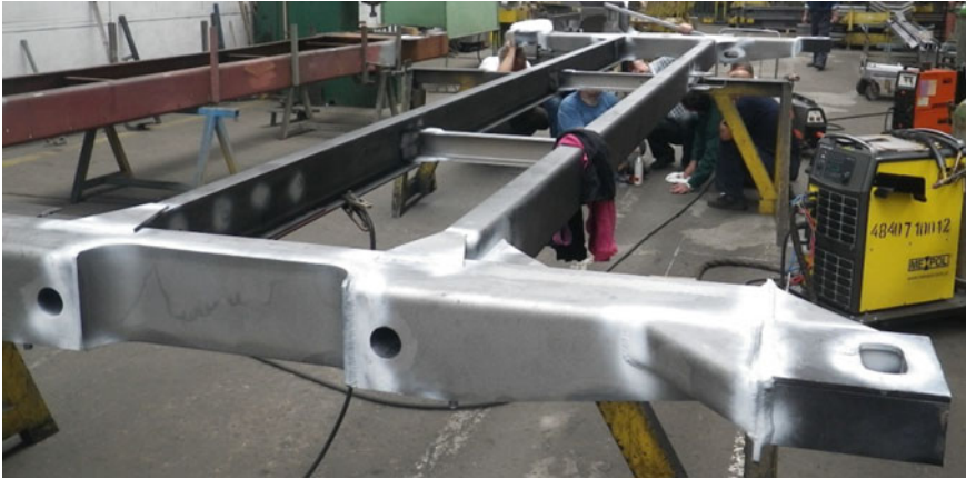
Fig. 12 Container-supporting frame—inspection of weld joints
