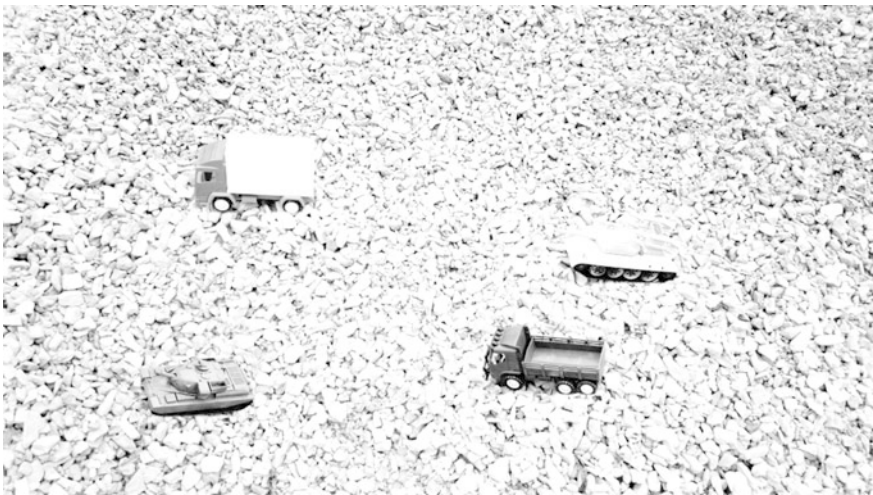
Fig. 8 The whole image of the terrain where the recognised objects are moving obtained after histogram equalisation according to grey levels obtained for the object 4
