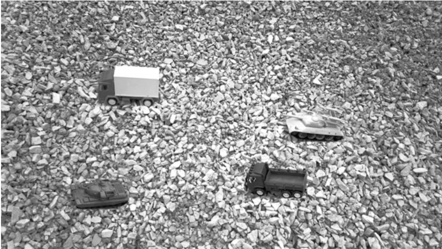
Fig. 5 The whole image of the terrain where the recognised objects are moving obtained after histogram equalisation according to grey levels obtained for the object 1
