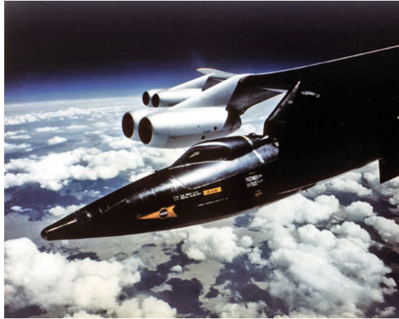
Fig. 6 Like SpaceShipOne and SpaceShipTwo, the X-15 was launched from a mother ship, in this case a B52 strategic bomber
