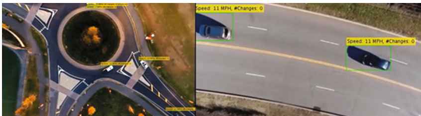
Fig. 5. Speed detection algorithms tested on real footage
