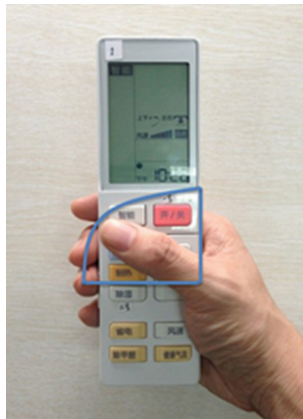
Fig. 6. Remote controller: an application of the thumb's comfortable control area
