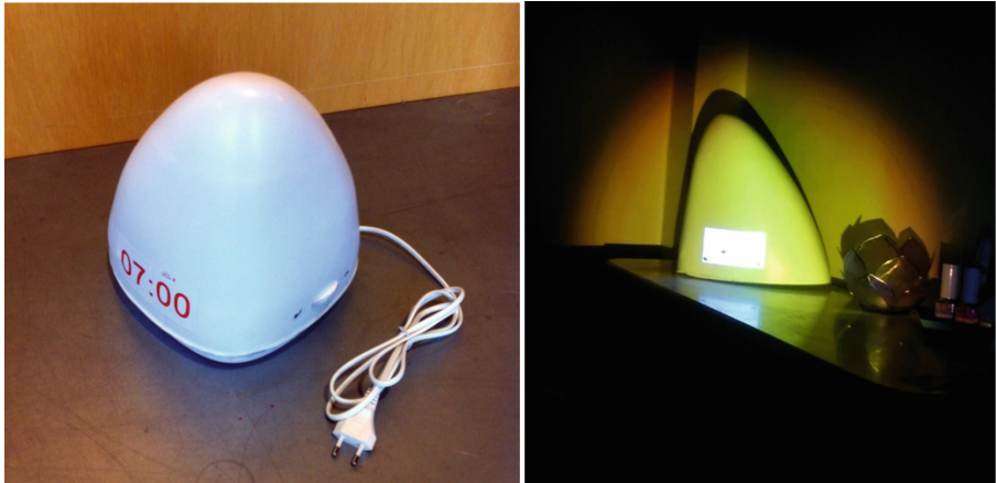
Fig. 5. Physical mock-up of the ‘wake up’ light project, augmented with Dynamapper to show the intended interface and light glow.
