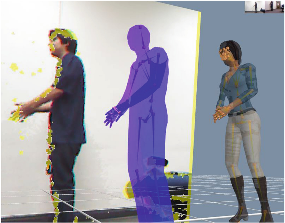
Fig. 2. From left to right, video and depth noise from the participant, motion capture data, and agent with animation data incorporated. The top right displays a thumbnail view of the raw front and side video as processed with iPi Soft.
