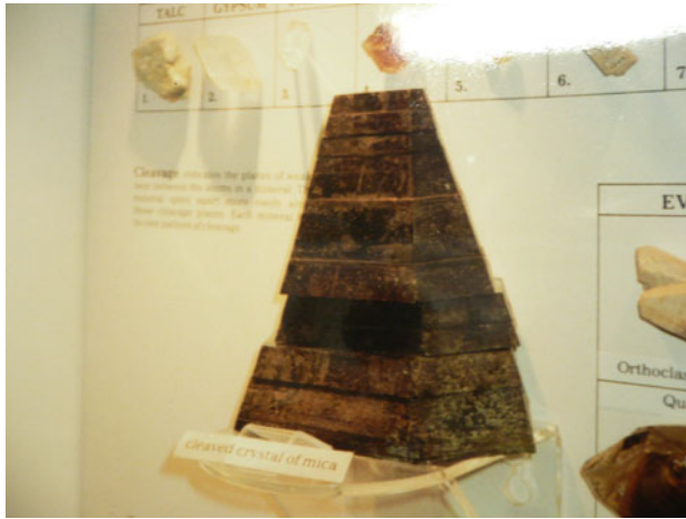
Fig. 20.5 The frontispiece showed a cluster of small crystals of mica. The photo shows a large well formed crystal of muscovite mica. It has been broken along the easy cleavage plane in several places during its extraction from the rock in the mine. It is about 60cm high. It is on display in the mineral section of the Australian Museum in Sydney
