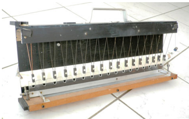
Fig. 20.23 Photograph of the arrangement of pendulums made from wire with permanent magnets attached at the bottom to form a linear chain of interacting magnets
