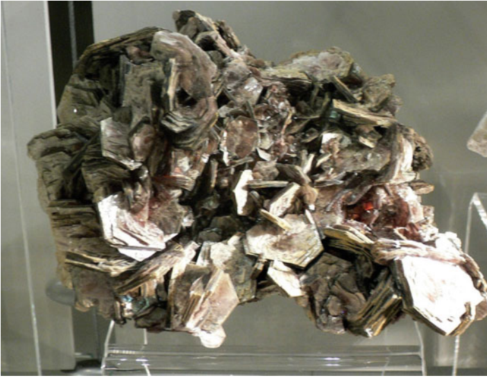
Fig. 20.1 A near life-size cluster of mica crystals, showing their layered nature and hexagonal habit. These crystals are too small and contain insufficient amounts of impurities to show the dark lines found in larger crystals
