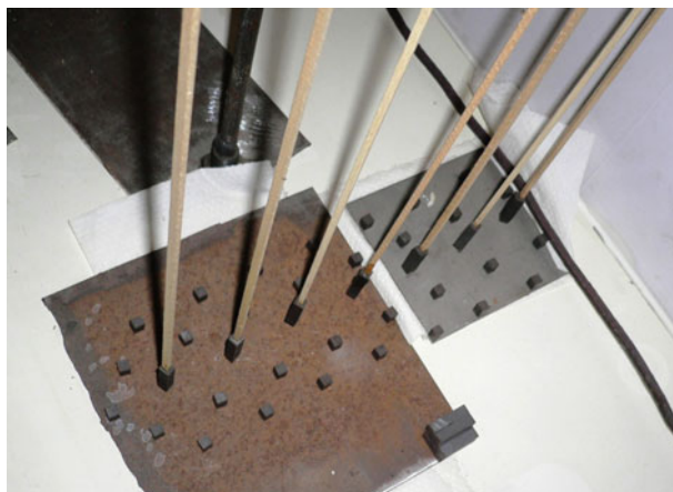
Fig. 20.22 This shows the first mechanical analogue of a chain of permanent magnets suspended at the bottom of long rigid sticks to simulate the behaviour of a chain of atoms. The sticks are attached at the top to a rigid fixture by means of cotton threads of 5 mm length. The suspended magnets rest in potential energy wells created by an array of magnets attached to a steel base plate. This analogue was used to study the behaviour of a chain of particles with nonlinear repulsive forces when disturbed by an external impulse to one magnet. It demonstrated the focussing action first postulated by Silbee in 1957
