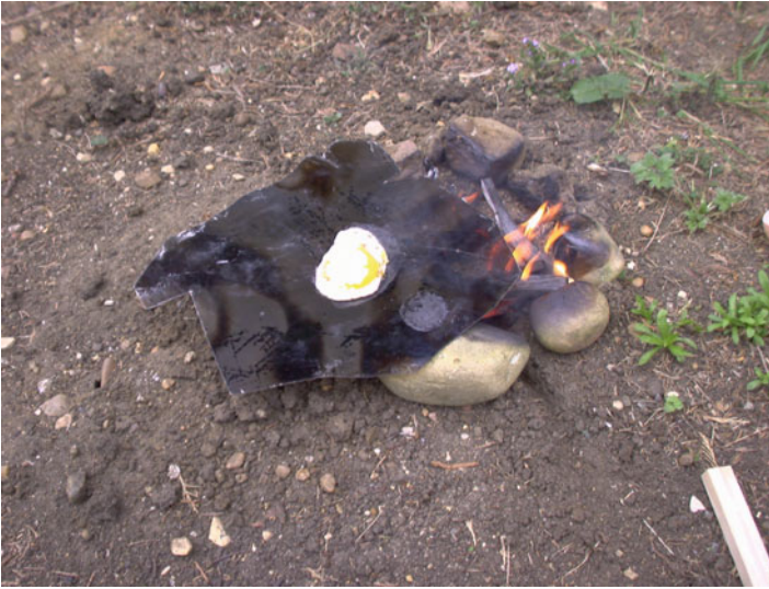
Fig. 20.7 Cooking an egg on a sheet of mica. The flames from below cause the sheet to buckle into a saucer shape, in which liquids can be poured. The sheet is about 210 mm × 200 mm × 1/5 mm thickness. It can be used more than a hundred times if handled carefully
