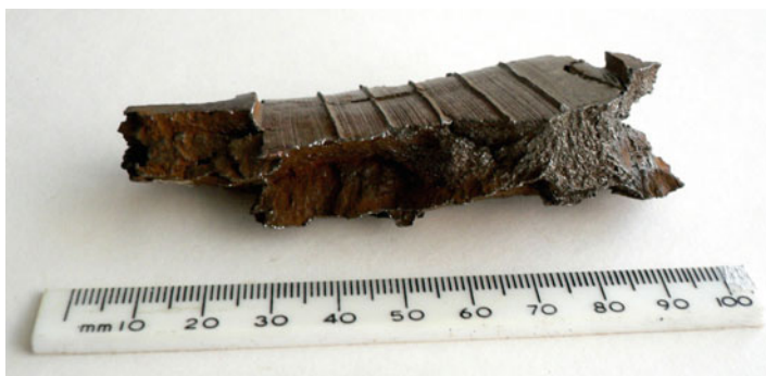
Fig. 20.2 A piece of shrapnel from anti-aircraft shells that fell near the author when he was running home from school during the Battle of Britain in 1940. Small crystals were visible in the fractured metal
