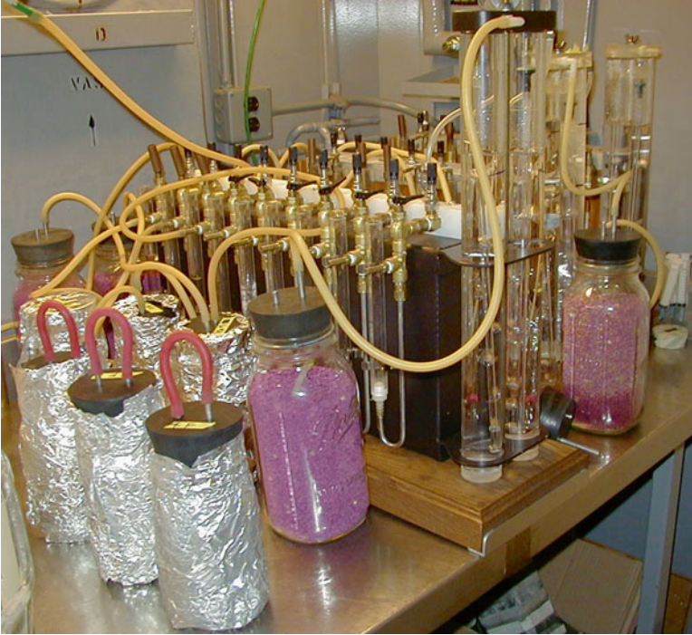
Fig. 5.9 Manifold system for regulating and distributing dilute ethylene gas mixtures into experimental jars in a walk-in environmental chamber in the Post-Harvest Laboratory of the Department of Pomology at the University of California in Davis, CA, USA
