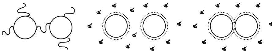
Fig. 8.2 Left: Schematic representation of bridging flocculation; one molecule attaches to two or more droplets due to insufficient surface coverage. Middle and right: illustration of depletion flocculation by non-adsorbing component. This component will have a non-accessible area near the droplets (indicated by the dotted line ) that corresponds to the gyration radius of the component, and because of that, there is an osmotic pressure difference that may lead to aggregation (see text for further explanation)
