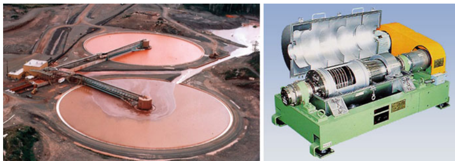
Fig. 10.3 A view of two thickeners showing the central driveheads which drive submerged rotating arms ( left , Courtesy of Dorr-Oliver Eimco) and a vane decanter centrifuge with the motor drive and gearbox being visible at the right hand end of the unit ( right , Courtesy of Mitsubishi Kakoki Kaisha)
