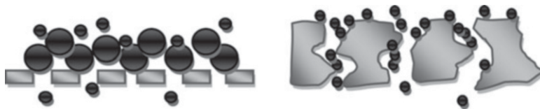
Fig. 12.1 Sketch of surface filtration ( left ) and depth filtration ( right )
