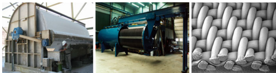
Fig. 10.1 A 92 m 2 roller discharge rotary vacuum filter ( left , Courtesy of Dorr-Oliver Eimco) and a vertical leaf pressure vessel filter ( middle , Courtesy of LFC). Micrograph of a typical woven filter medium ( right , Courtesy of Sefar)
