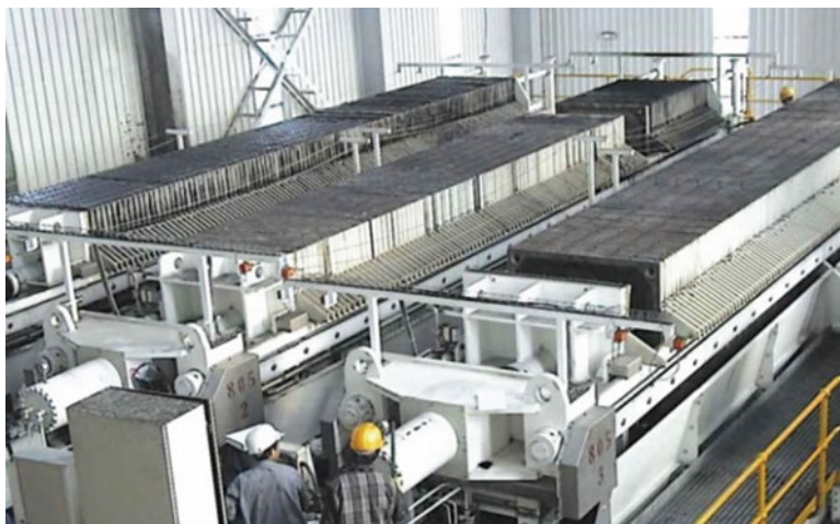
Fig. 10.11 A sidebar diaphragm press installation (Copyright © Outotec)
