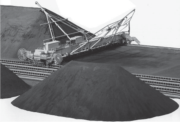
Fig. 9.7 Recovery of the fine homogenized coal by system Chevron (Central Coking Plant Saar GmbH, Germany); width of the bridge scraper: 57.5 m; capacity 1200 t/h; (Courtesy PWH – Krupp Engineering)
