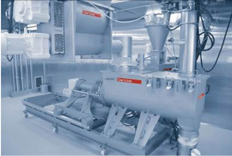
Fig. 9.15 Continuous mixing for the production of milk powder mixers: Continuous gravimetric solids feeder (loss-in-weight feeding) supply at constant rate the components (base powder and micro ingredients) directly to the continuous mixer (Courtesy Gericke AG)
