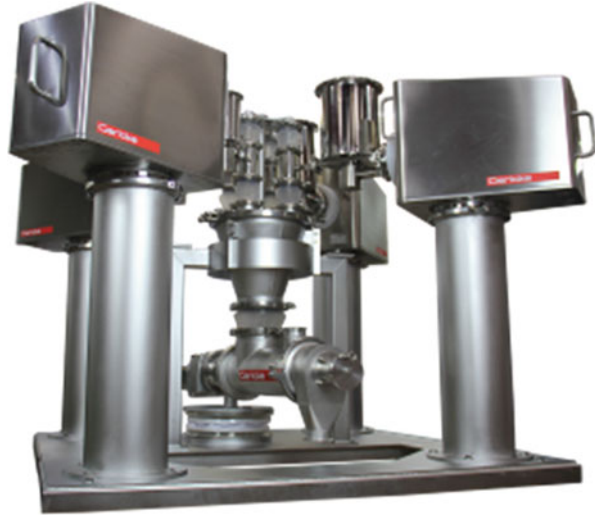
Fig. 9.17 Continuous feeding and mixing installation for pharmaceutical ingredients. These elements are used for continuous manufacturing production upstream direct compact, dry or wet granulation and hot melt extrusion (Courtesy Gericke AG)
