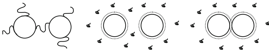
Fig. 8.2 Left: Schematic representation of bridging flocculation; one molecule attaches to two or more droplets due to insufficient surface coverage. Middle and right: illustration of depletion flocculation by non-adsorbing component. This component will have a non-accessible area near the droplets (indicated by the dotted line) that corresponds to the gyration radius of the component, and because of that, there is an osmotic pressure difference that may lead to aggregation (see text for further explanation)
