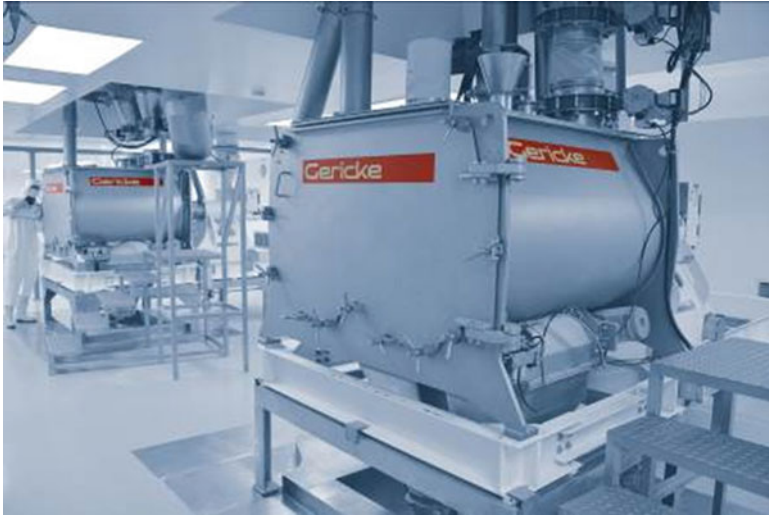
Fig. 9.13 Batch mixing installation for nutritional products. Hygienic design principles have been applied to minimize the risk of cross contamination between batches (Courtesy Gericke AG)
