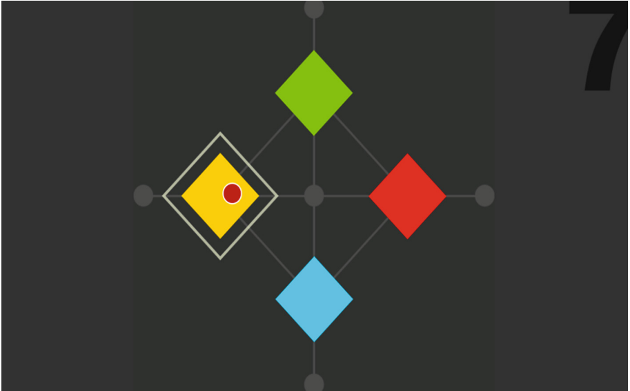
Fig. 1. A screenshot of the gaze enabled Simon game. The colorful squares are the objects of the game. The red circular dot represents a user's gaze point during the gameplay. To activate an object (e.g., the yellow square in the above scenario) the player has to directly look at the target object (Color figure online).
