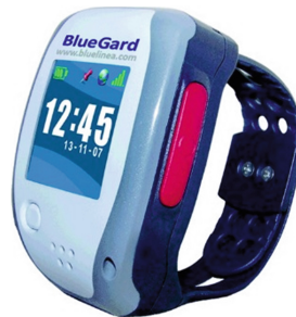
Fig. 2. The “BlueGard” bracelet for monitoring the location of persons with dementia
