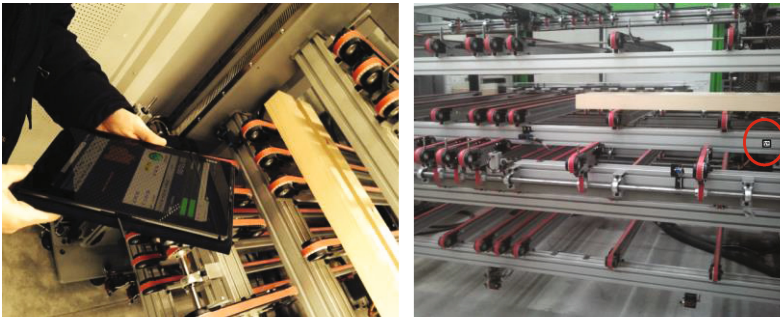
Fig. 5. Experimentation: AR application reading the marker positioned on the machine tool
