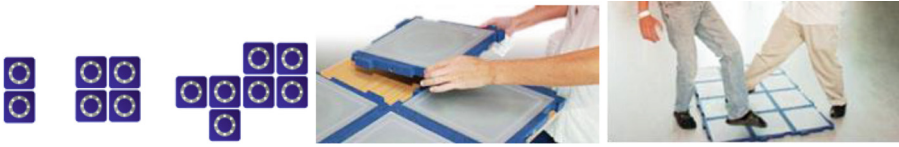
Fig. 2. The modular interactive tiles can be assembled in different configurations for different playful exercises and levels.
