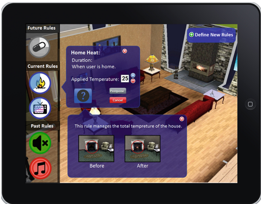
Fig. 3. The proposed meta user interface provides an image of Ambient Intelligence meta systems. It is designed to support visibility, predictability, overriding default behavior, conflict handling, and perceived control in presence of system initiated automated behaviors (implicit interaction).
