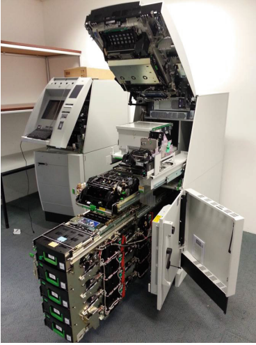
Fig. 1. Internal components of a Wincor Nixdorf CINEO 4060 Cash Recycling Machine.
