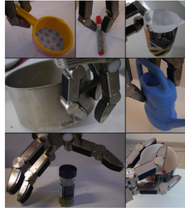
(b) Grasps executed using learned task constraints. Handle, cork, pouring, and lift up.
