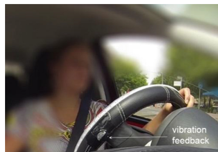
Fig. 4. The haptic (vibration) feedback
