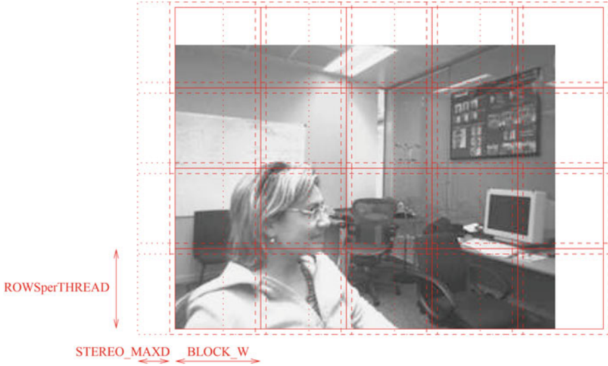
Fig. 8.8 The left and right images (solid rectangle) are split into BLOCK\_W \times ROWSperTHREAD tiles. The dashed lines indicate the extra pixels outside the tile which must be read to calculate values for pixels in the tile. The right hand image is progressively offset by between zero and STEREO\_MAXD pixels (50, dotted lines)
