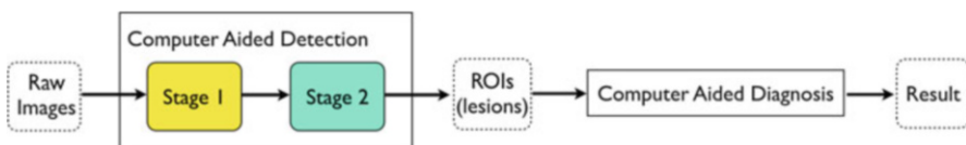
Fig. 10.3 A typical flowchart for computer aided detection and diagnosis. Stage 1 of the process aims to detect suspicious areas with high sensitivity, while Stage 2 tries to reduce the number of suspicious lesions without compromising sensitivity
