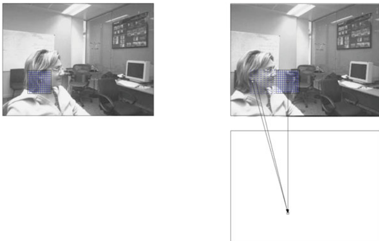
Fig. 8.7 Schematic of stereo disparity calculation. Top: left and right stereo images. Bottom: output. Not to scale. For each pixel stereoKernel calculates the sum of squared differences (SSD) between 11 \times 11 regions centred on the pixel in the left image and the same pixel in the right hand image. This is the SSD for zero disparity. The right hand 11 \times 11 region is moved one place to the left and new SSD is calculated (SSD for 1 pixel of disparity). This is repeated 50 times. Each time a smaller SSD is found, it is saved. Although the output pixel ( bottom ) may be updated many times, its final value is the distance moved by the 11 \times 11 region which gives the smallest SSD. That is the distance between left and right images which gives the maximum similarity between them (across an 11 \times 11 region). This all has to be done for every pixel. Real time performance is obtained by parallel processing and reducing repeated calculations
