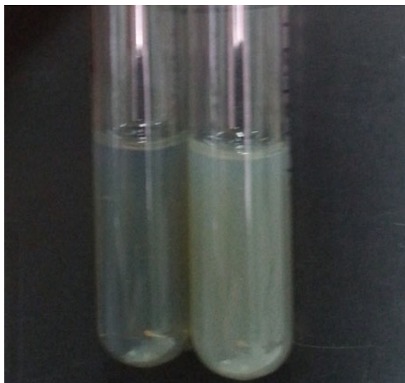
Fig. 8.10 Photo of the ND hydrosol coagulated by NaOH (right) and the same hydrosol after restoration via HCl (left). The final NaCl concentration formed after neutralization of the alkali was below the CCC value of NaCl
