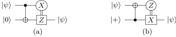
Fig. 3. Circuits for teleporting the state of a source qubit to a neighbouring destination qubit
