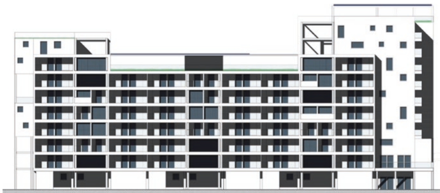
Fig. 8.31 New residential units both on the south and north sides of block building B6 combined with add-ons and new façade solutions in the existing residential units
