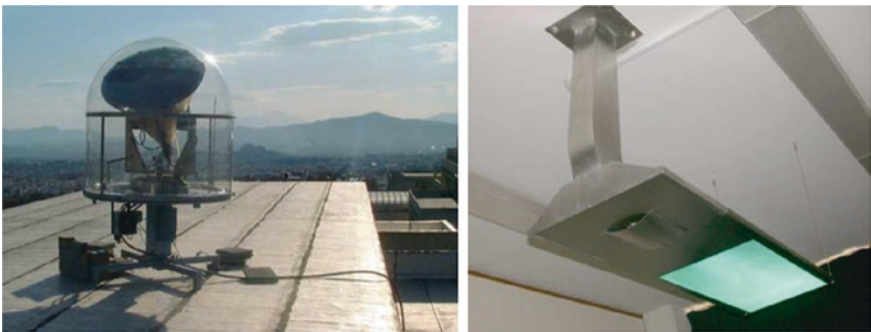
Fig. 21.29 Solux system tested during Universal Fiber Optics project
