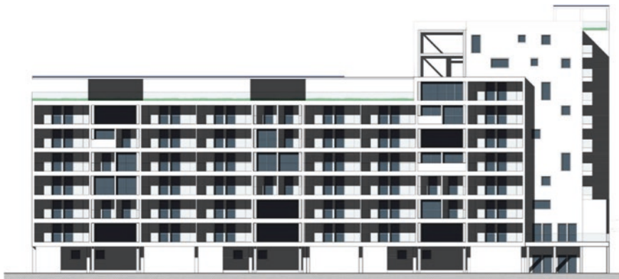
Fig. 8.30 New residential units on the south side of block building B6 combined with add-ons and new façade solutions in the existing residential units
