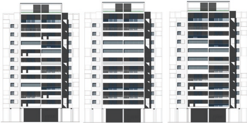
Fig. 8.28 Combination of additions on the top (new residential units) and on the elevation of the buildings with new façade solutions selected from the abacus for the north and west façades in the tower typology
