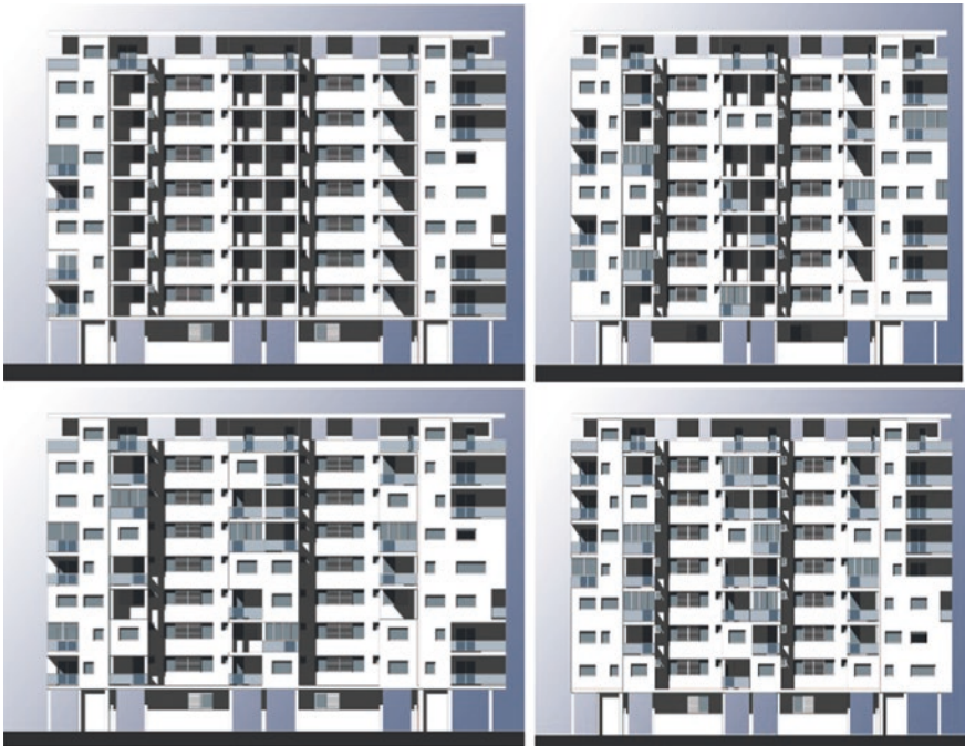
Fig. 8.33 North façade of Block T7: new residential units combined with add-ons and new façade solutions in the existing residential units
