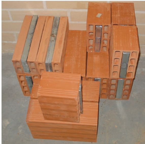
Fig. 16.10 Clay bricks including PCM macrocapsules (Kuznik et al. 2008a, b)
