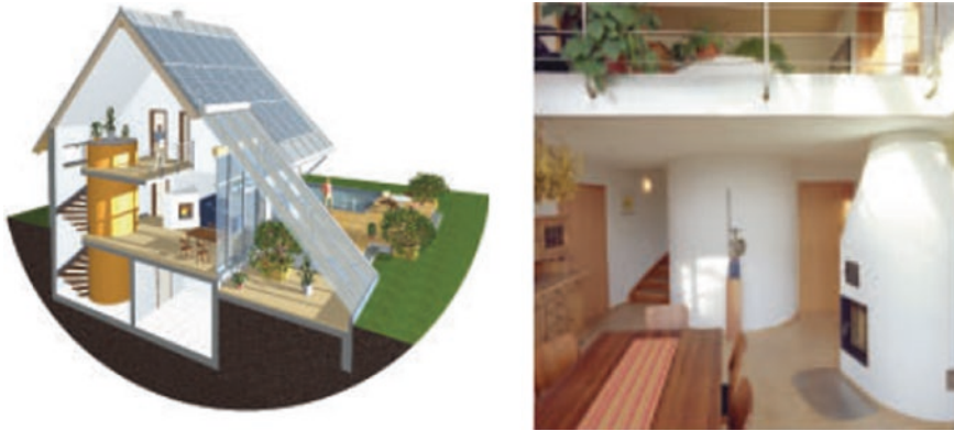
Fig. 16.20 Solar water tank integrated in a living room (Solaresbauen-Grundlagen 2014)
