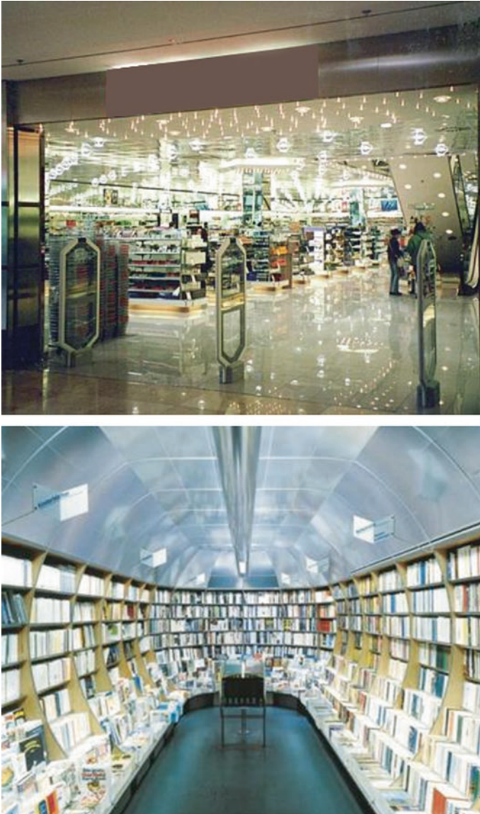
Fig. 22.12 Comparison of shop lighting (at left , the light points are the focus; at right , the wares)
