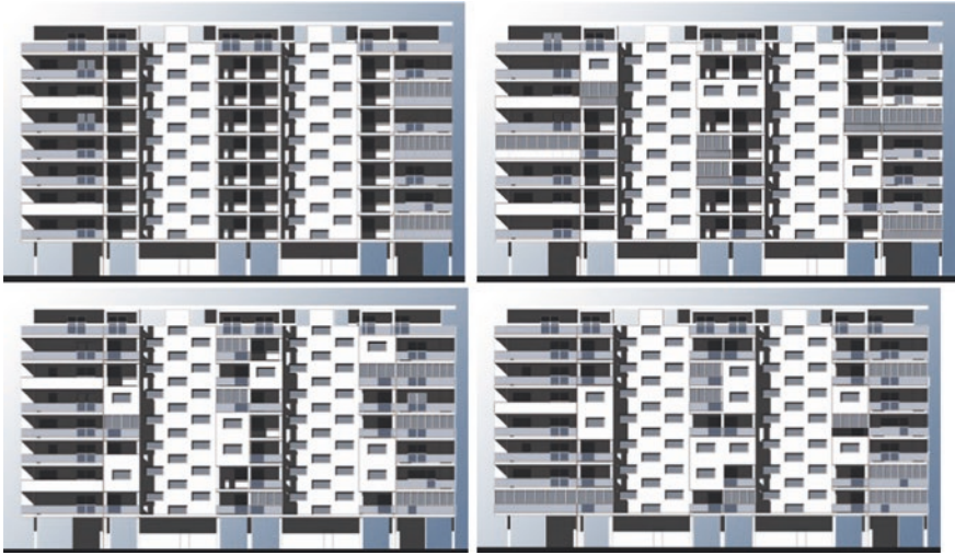
Fig. 8.32 South-oriented façades of the Block T7: new residential units combined with add-ons and new façade solutions in the existing residential units
