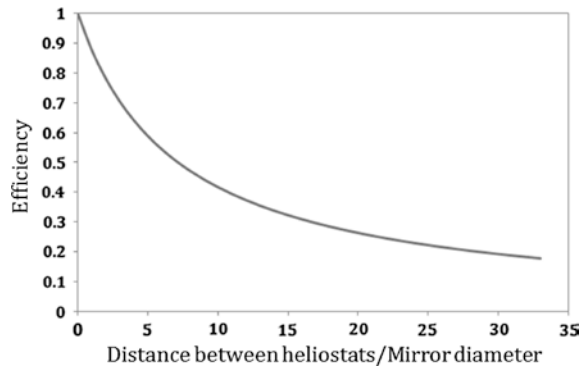
Fig. 21.31 Sunlight transmission efficiency when a heliostat and a same-size static mirror are used
