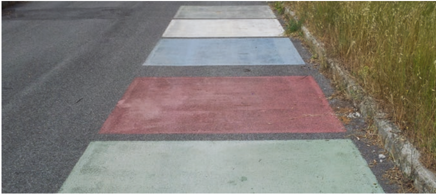
Fig. 20.8 Different chromatic versions of a commercial coating for road pavement. Noteworthy is the effect of the cool pigment, which gives an NIR reflectance higher than the luminous reflectance up to a factor 4 (for the green and the red samples); increments are limited for the lighter colors. One of the best performing coating for pavements has an 83 % NIR reflectance and 23 % light reflectance
