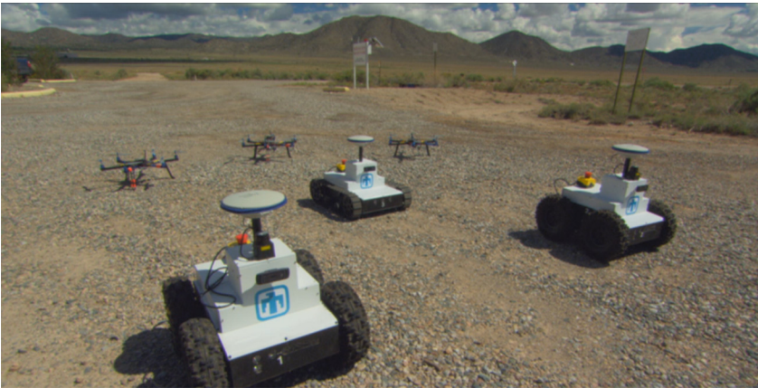
Fig. 5. UGVs and UAVs for SAHUC's proof-of-concept implementation
