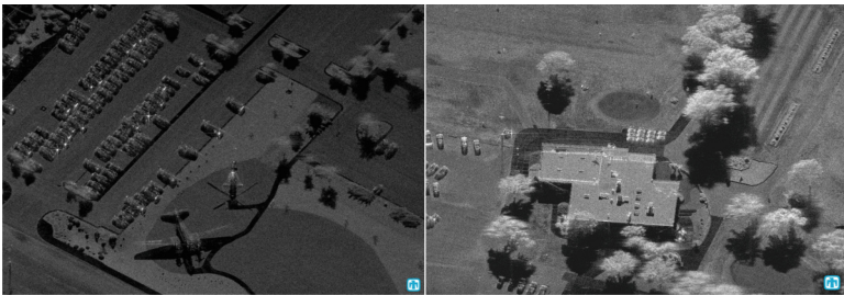
Fig. 4. Synthetic Aperture Radar (SAR) images of a static display of a helicopter and plane (left) and of the Kirtland Air Force Base golf course clubhouse (right). Images are courtesy of Sandia National Laboratories, Airborne ISR ( http://www.sandia.gov/radar/imagery/index.html ).
