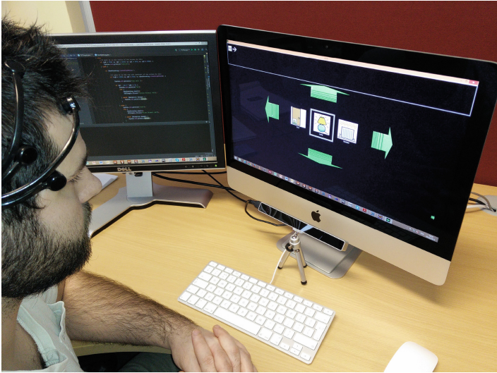
Fig. 1. The IGUI interactive menu system facilitates domotic control within a smart environment. Navigation through levels of an event hierarchy is conducted through 4-way directional control. A distinct event or current level is positioned in the centre of the interface.
