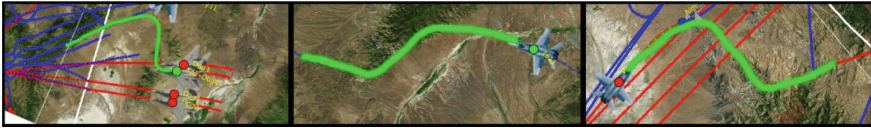
Fig. 5. Sections of flight paths that, to varying degrees, resemble an ideal beam maneuver in which the aircraft turns to place an oncoming threat directly to the left or right. TAF assigned a match quality of 99 % (left), 55 % (middle), and 34 % (right).
