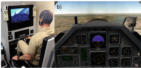
Fig. 2. A flight simulation task; (a) EEG, ECG, and flight data were monitored while the subjects were engaged in the task. (b) the main instrument console in virtual cockpit contains all instrumentation and systems displays for the aircraft. The cockpit layout is based on the US air force and navy joint primary aircraft training system training documentation.
