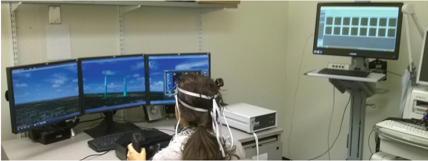
Fig. 5. Subject operating the C-130j simulator with fNIR sensor attached and data acquisition apparatus on far right.
