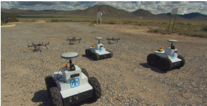
Fig. 5. UGVs and UAVs for SAHUC's proof-of-concept implementation
