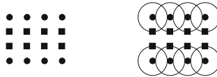
Fig. 3. PSF illustration with Grid Line; ( Left ) Input point grid (i.e., pixels); ( Right ) Perceived image; squares represent “grid pixels”. Note that each “grid pixel” has a minimum of three adjacent “correction pixels”.
