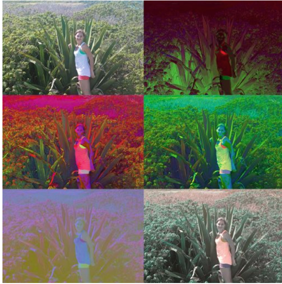
Fig. 1. The same image encoded in six different colors spaces, saved in JPEG, and displayed by using IrfanView. In the first row, the image in sRGB and the scaled difference image between sRGB and AdobeRGB, HSV and HLS (second row), and Lab and XYZ (third row)(Color figure online).
