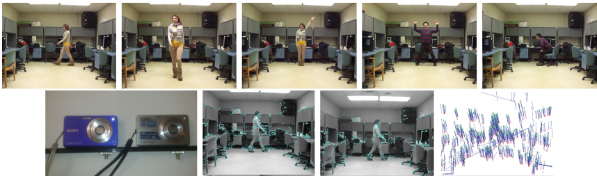
Fig. 1. First row: Sample frames of five different activities, Second row: Cameras used, the left and right extracted feature points and their matching result
