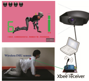
Fig. 3. Overview of VR-based LBP rehabilitation system
