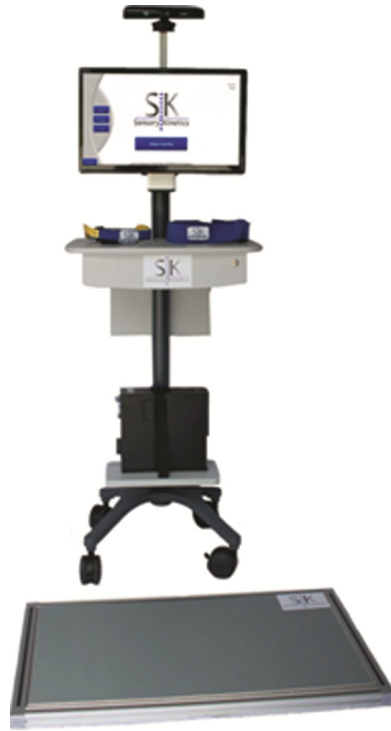
Fig. 2. Multimodal balance rehabilitation training device showing the force plate, Microsoft Kinect camera and wearable inertial sensors, together with the touch screen and tactile belt.
