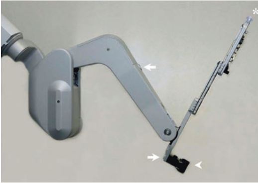
Fig. 2.7 Photograph of the da Vinci® S instrument arm including the port clutch buttons (arrows), showing camera/instrument clutch buttons (arrows) and trocar mount (arrowhead)
