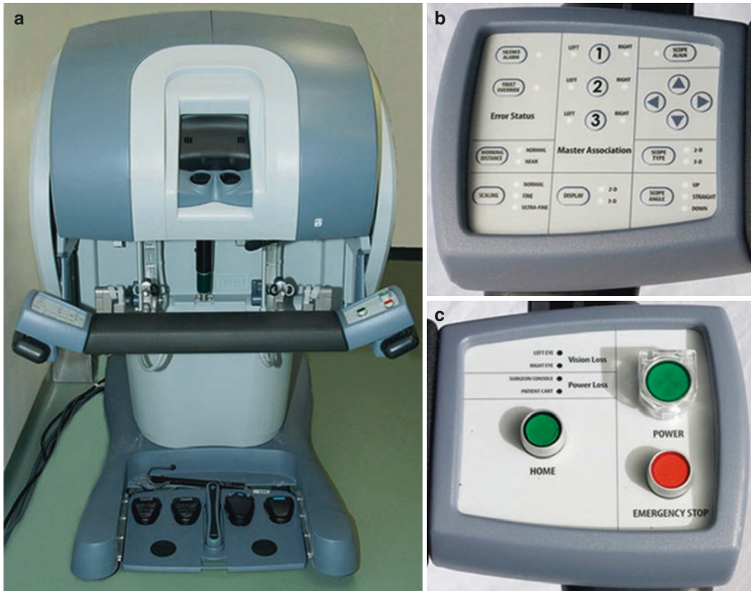
Fig. 2.1 Photograph of da Vinci® S and S-HD surgeon console (a) and side pod controls (b, c)
