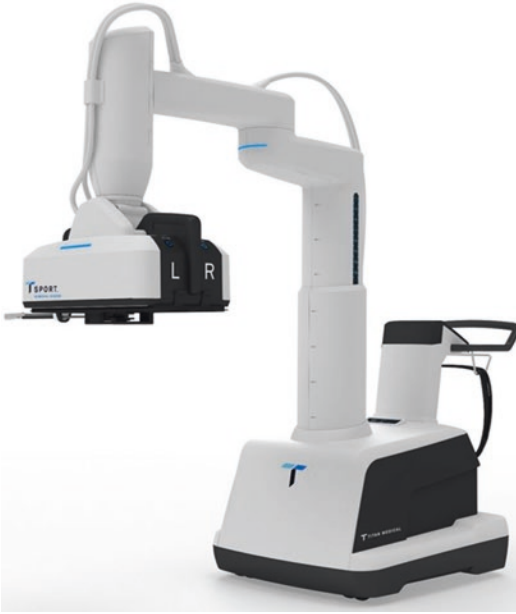
Fig. 70.1 The patient cart of SPORT system (With permission from Titan medical Inc.)
