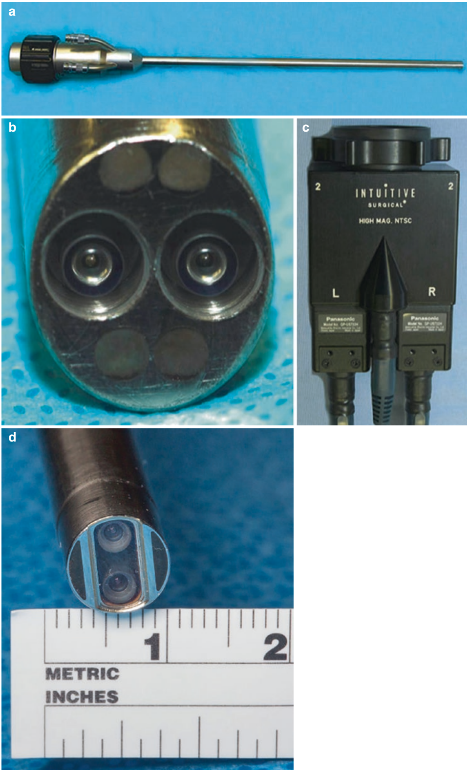
Fig. 2.3 Photograph of the da Vinci® stereo endoscope (a) showing the two individual 5-mm endoscopes (b) and camera (c) with right and left optical channels, as well as the new da Vinci® Xi stereo endoscope with updated optics (d)
