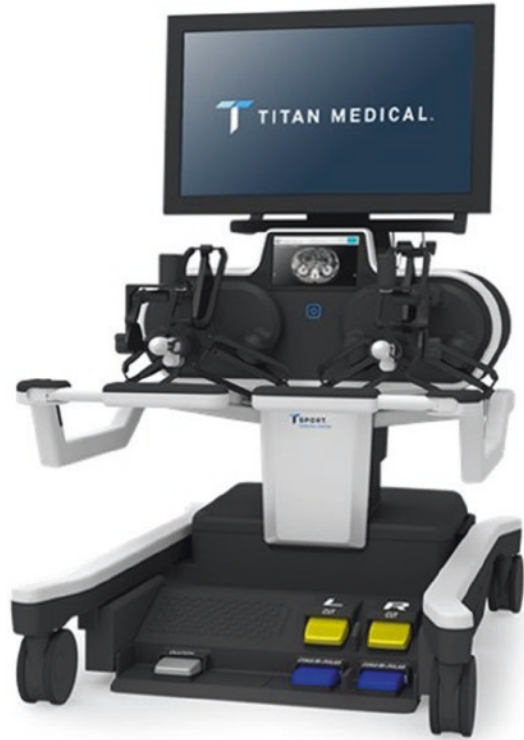
Fig. 70.2 The surgeon console of SPORT system (With permission from Titan medical Inc.)
