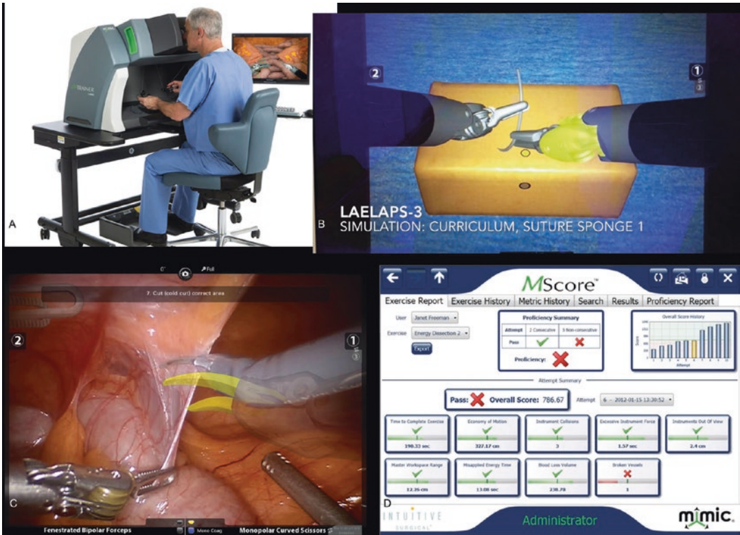
Fig. 14.1 Mimic dV-Trainer and exercises. (a) dV-Trainer console. (b) Suturing exercise. (c) Maestro Augmented Reality. (d) Example score report. (Used with permission from Mimic Technologies, Inc.)
