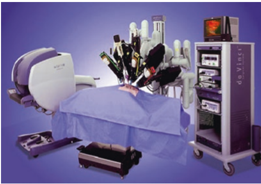
Fig. 8.1 Three components of the da Vinci robot – surgeon console, patient-side cart, and vision tower
