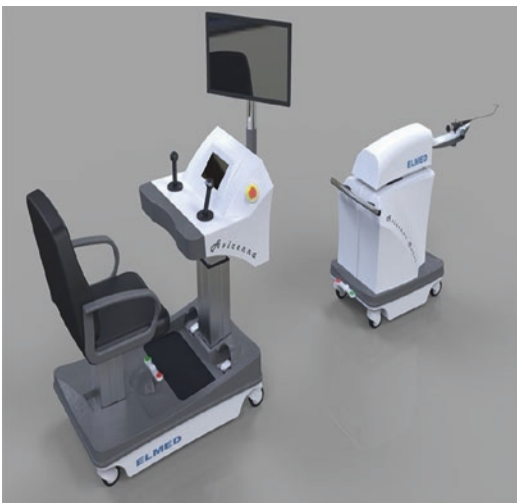
Fig. 70.4 The patient cart and surgeon console of Avicenna roboflex flexible ureteroscopy robot (With permission from ELMED)
