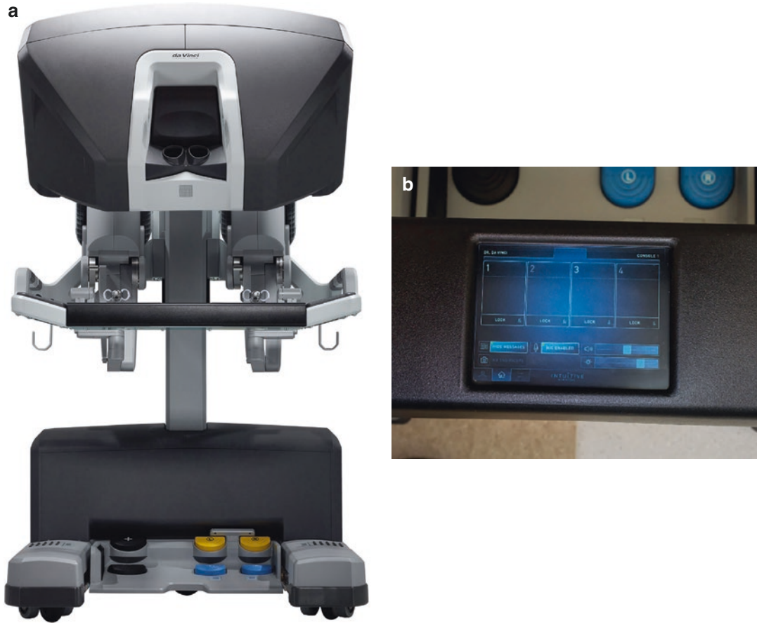
Fig. 2.2 Photograph of da Vinci ® Xi system with surgeon console (a) and center touch-pad (b). (Reproduced with permission from Intuitive Surgical; Inc© 2017 Intuitive Surgical, Inc.)
