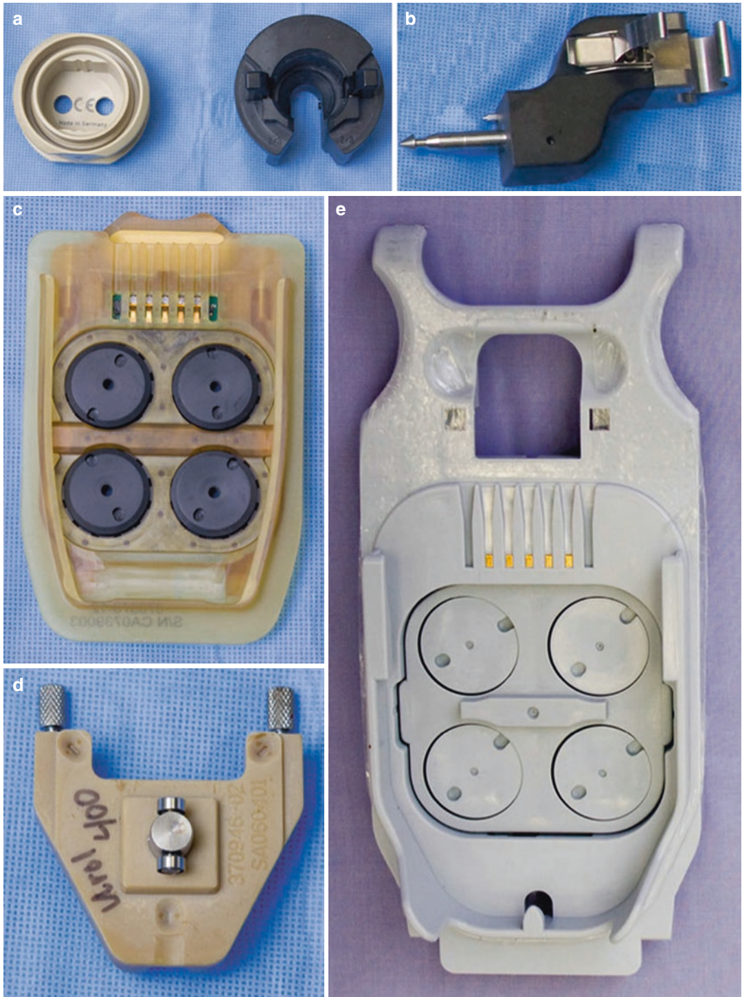
Fig. 2.8 Photographs of sterile accessories placed during the draping procedure. (a) Camera sterile adapter (left) and camera arm sterile adapter (right) and camera trocar mount (b). da Vinci® standard instrument arm sterile
