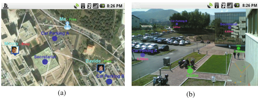
Fig. 2. (a) MapMode visualization of POIs and users’ position. (b) LiveMode representation of a user’s position.
