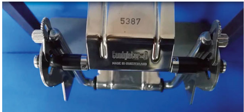
Fig. 13.7 The articular mechanism of the Gerber Condylator. The pure lateral movement (Bennett movement). Upper view (Video 13.3)
