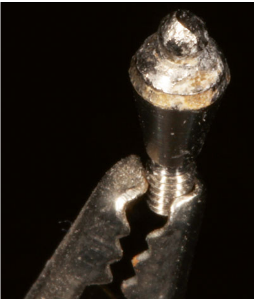
Fig. 20.52 In case of wear of the implant abutments, it is also necessary to change the abutments
