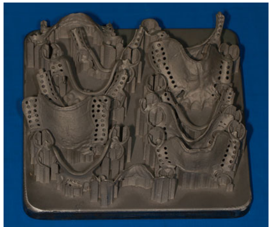
Fig. 14.32 Metal frameworks produced by laser sintering
