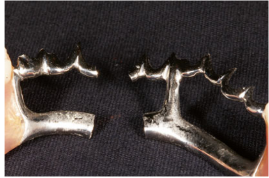
Fig. 20.24 Kennedy bar may weaken after some time, and the weakened parts cannot tolerate intraoral stresses and may break
