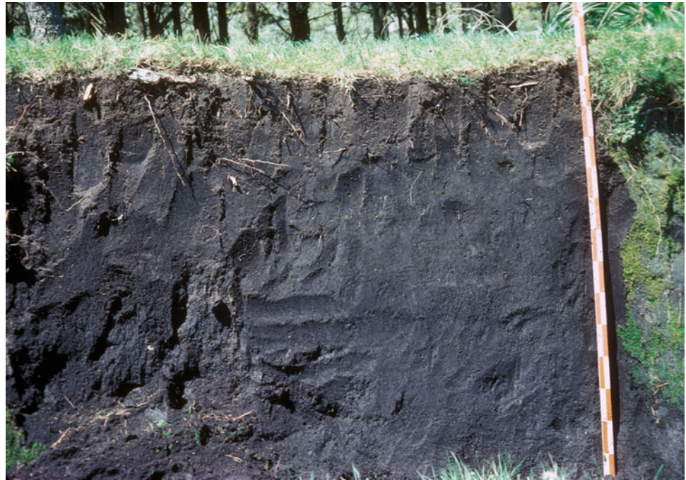
Fig. 3.61 Umbric Melanic Andosol (Dystric, Thixotropic) on granite of two micas. Monte Xiabre, Pontevedra, Galicia
