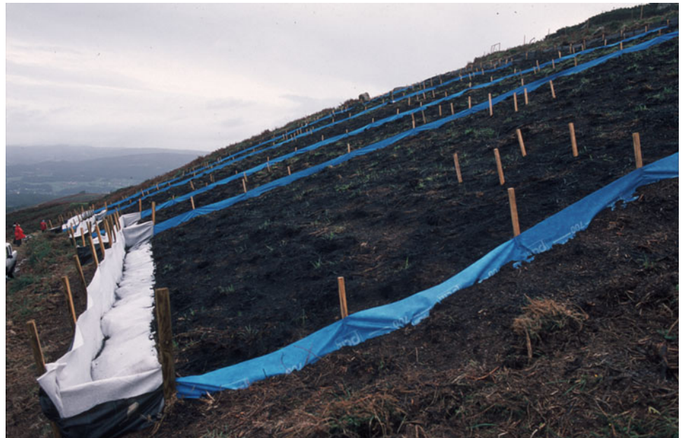
Fig. 3.36 Field experiment for evaluating two bioremediation techniques, seeding and mulching (straw) for burnt soil protection, erosion control (by geo-textile fences) and ecosystem rehabilitation (Orense, Galicia)
