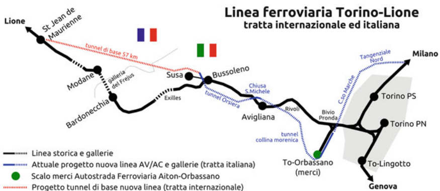
Fig. 6.4 Current design of the TAV line connecting Turin and Lyon; the new route shows the 57 km long tunnel and the inclusion of the Orbassano station.
