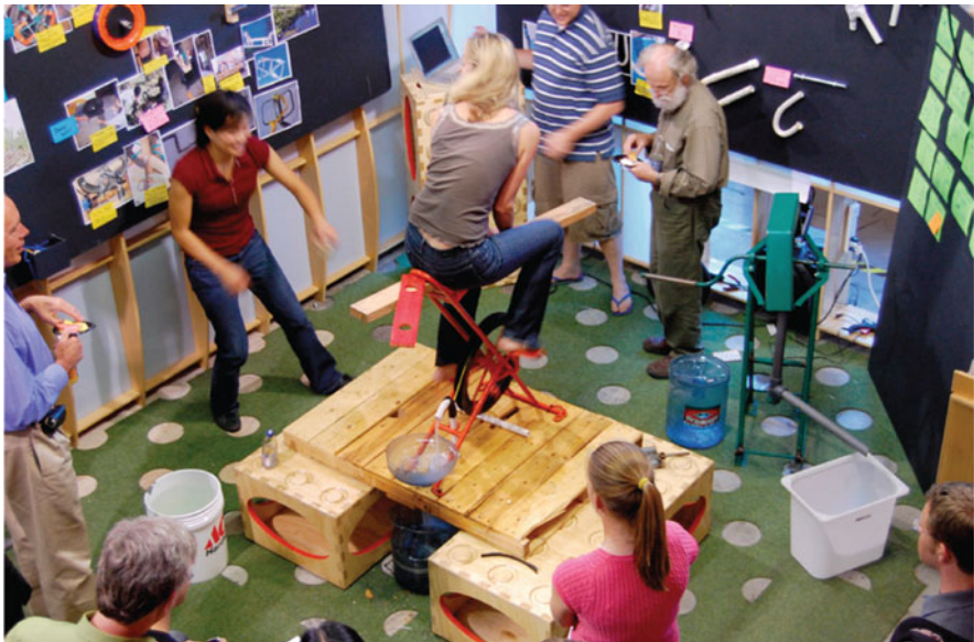
Fig. 9.5 A rapid prototype of a human-powered pump being tried out by students. Photo credit: d.school
