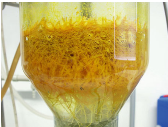
Fig. 1 Hairy roots of Devil's claw ( Harpagophytum procumbens ) in a bubble column bioreactor [16]
