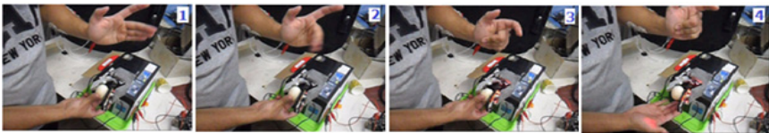
Photos. 2. The clamp holding a raw egg. The egg was taken by horizontal sides successfully, without any damage, the test was repeated any the results were the same.
