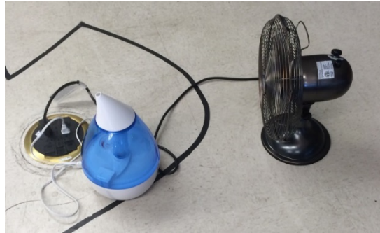
Fig. 5. The experiments on moth-inspired plume tracing under turbulent airflow environments are conducted by the plume tracer. A humidifier pumps alcohol as the chemical source and a fan with a fix heading or a varying heading is used to generate turbulent airflow.
