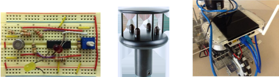
Fig. 2. The electrical circuit board for the Figaro chemical sensor converts chemical concentrations into electrical output signals (left). The Gill WindSonic sensor is a low-cost anemometer, which provides wind speed and direction data via one serial or two analogue outputs (middle). A wireless router integrated on the DaNI robot is for wireless communication between a computer and the DaNI robot (right).
