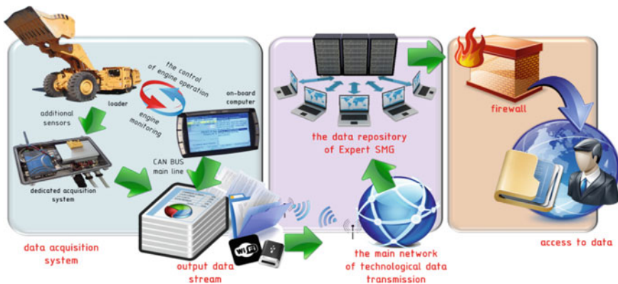
Fig. 1 Functional flow chart of the decision support system can be categorized following 3 layers. a Data acquisition, b data transmission, c data processing and presentation
