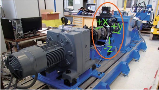
Fig. 3 A picture of the wind turbine test rig. The 3 accelerometers are represented by green arrows . The main bearing and its loading unit is circled in orange
