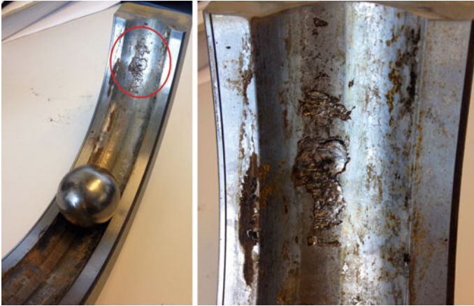
Fig. 10 Fault on the outer race
