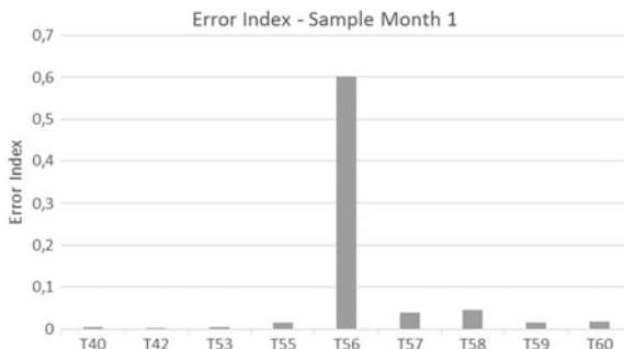
Fig. 2 Monthly test case 1: huge malfunctioning on turbine T56
