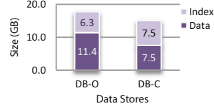
Fig. 1. Bulk-loading performance of 6 GB logs Fig. 2. Index and database size of 6 GB of logs
