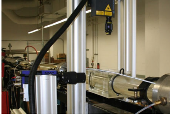
Fig. 3 The PIV setup consisting of a camera imaging perpendicular to the laser sheet. The test section of the flow loop is contained within a glycerol box minimizing distortion effects caused by the round glass pipe
