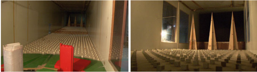
Fig. 2 General (left) and detailed (right) views of the wind tunnel test section and boundary layer preparation section, with roughness element cubes and vortex induction Standen spires type elements
