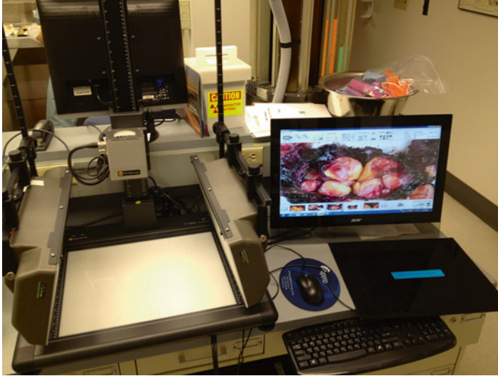
Fig. 6.1 Stand-alone contemporary macro imaging station (SPOT pathStation2) that can facilitate telepathology of large gross pathology specimens
