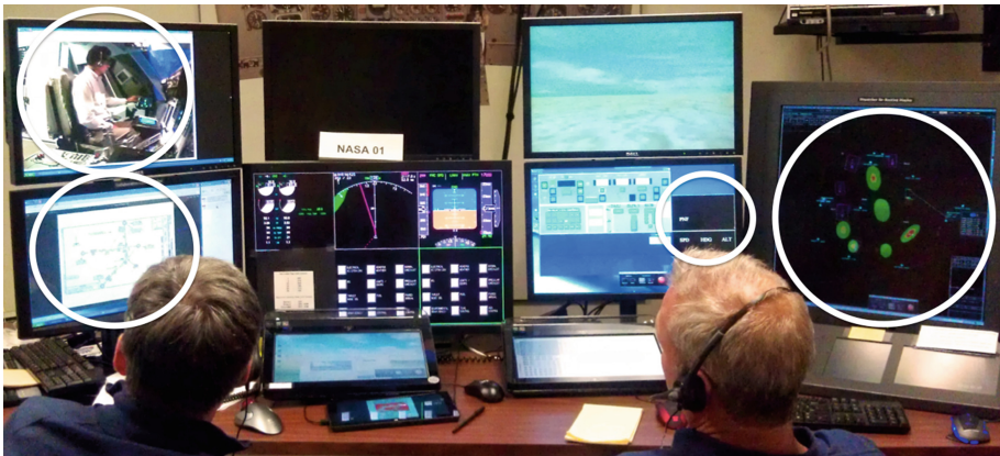
Fig. 2. In RCO with collaboration tool condition, the traffic and weather sector map (circled, far right) and the charts and approach plates display (circled, mid-left) can be shared with the captain, who is shown in the video feed (circled, upper left). Ground CRM indicators are to the left of the traffic and weather sector map. The ground operator shown is in CT training.
