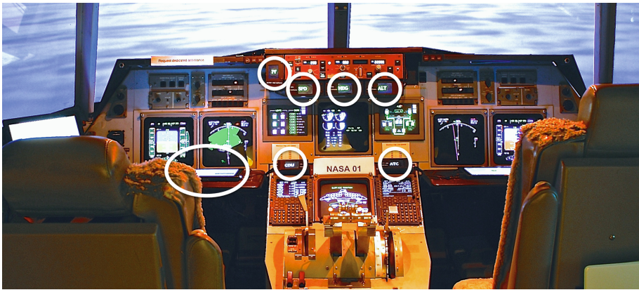
Fig. 1. Flight deck in RCO with collaboration tools condition. The six CRM indicators are mounted adjacent to their corresponding instrument panel. Captain’s EFB is circled to the left.
