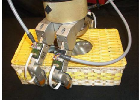
provides the feedback on the actual conditions and suggests a correction movement if necessary. A proper action for adapting the hand pose to the new situation can be computed from the difference between finger extensions. As represented in Fig. 6.19, any correction movement is made of two components:  $z$  for translation and  $\alpha$  for rotation.
