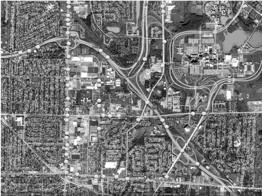
Fig. 8.3 Map of acoustic sensor location using explicit model strategy
