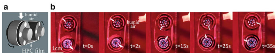
Fig. 14.4 Moisture-driven liquid crystal cellulose engine. (a) Schematic of the motor where it is possible to observe the directions of the moist air and rotation. (b) Sequence of video frames showing the motor performing work. Reprinted by permission from Macmillan Publishers Ltd: Scientific Reports, Geng Y, Almeida PL, Fernandes SN, Cheng C, Palfy-Muhoray P, & Godinho MH, “A cellulose liquid crystal motor: a steam engine of the second kind”. 3:1028, Copyright © 2013
