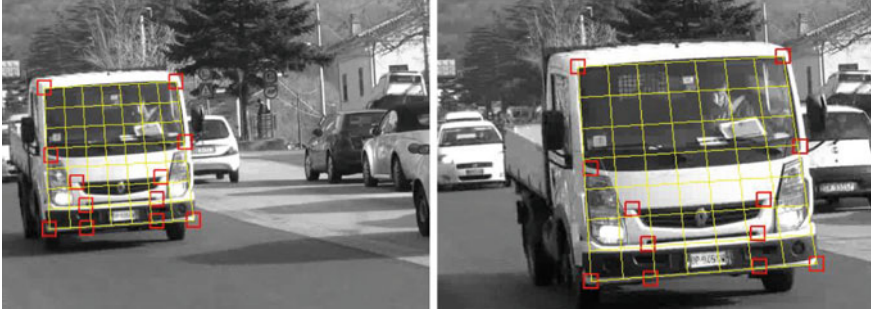
Fig. 9.1 Example of the CMBM algorithm applied to two frames of the sequence. The block matching is performed under the constraint that all blocks must maintain their relative positions
