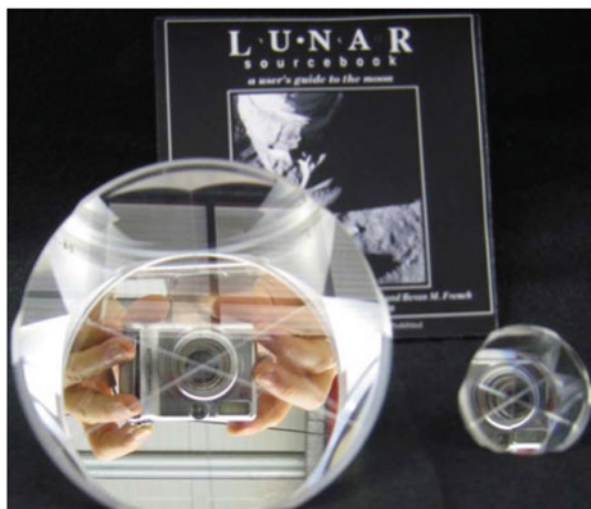
Fig. 2 Picture of Apollo, first generation and MoonLIGHT/LLRRA21, second generation CCR
