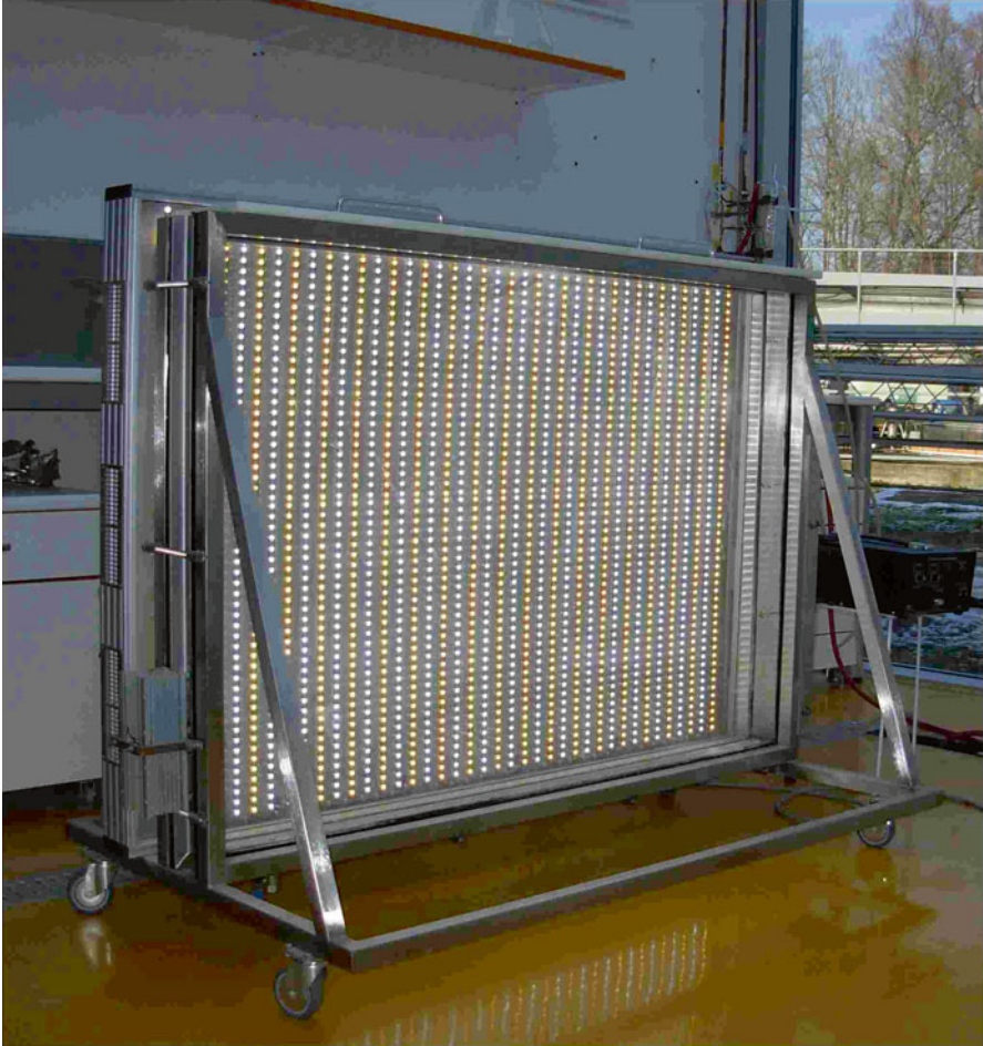
Fig. 3 An indoor flat-panel PBR for cultivation of microalgae with external illumination by light-emitting diodes (Institute of Microbiology, Třebo, Czech Republic). The PBR consists of a stainless steel frame holding glass plates; it has a volume of 80 L and has a short light path of 6 cm. The system is mixed by air bubbling (+1–2 % CO 2 ) and temperature is controlled by Peltier (thermo-electric) cells. The illumination panel consists of 2200 high-intensity white LEDs with adjustable light intensity. This PBR can generate the L/D cycles modulated in the microsecond scale (produced by Photon Systems Instruments Inc., Drasov, Czech Republic; http://www.psi.cz )
