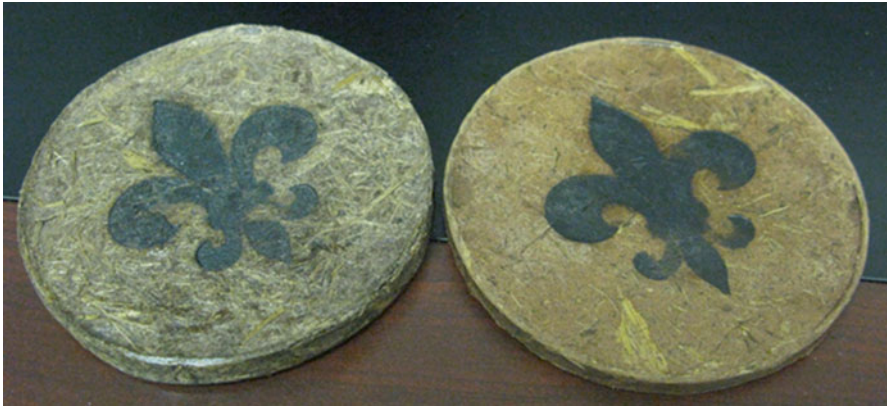
Fig. 4 Coasters made with algal glue binder. Coaster on left uses glue with sugarcane bagasse. Coaster on right also contains sawdust, resulting in a smoother surface
