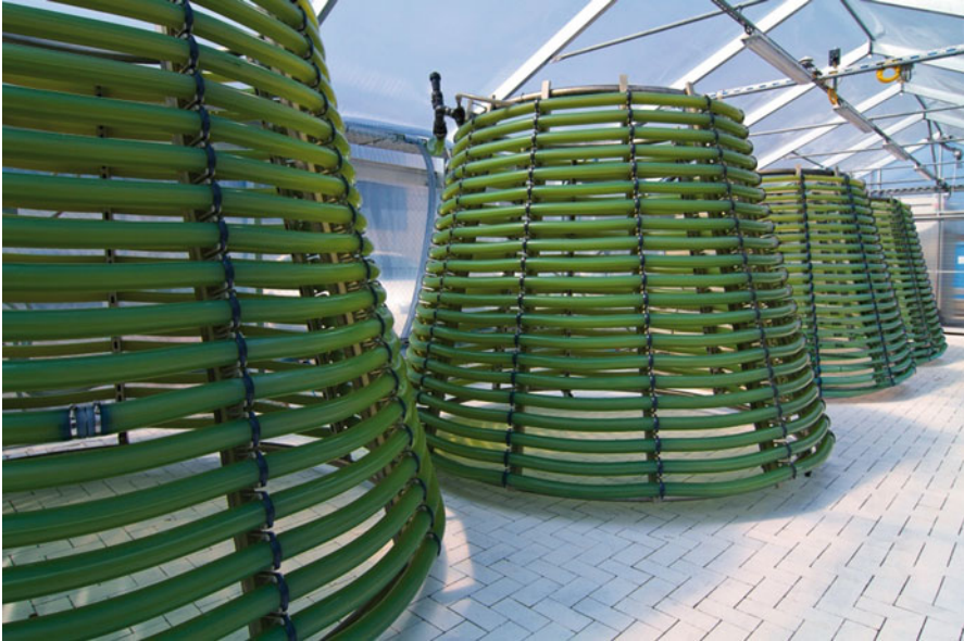
Fig. 22 The “Christmas tree PBR”, a conical variety of helical tubular PBRs (online resource 8, with kind permission from GICON – Großmann Ingenieur Consult GmbH). These examples are operated indoor in a glass house, using external solar illumination in addition to artificial internal illumination
