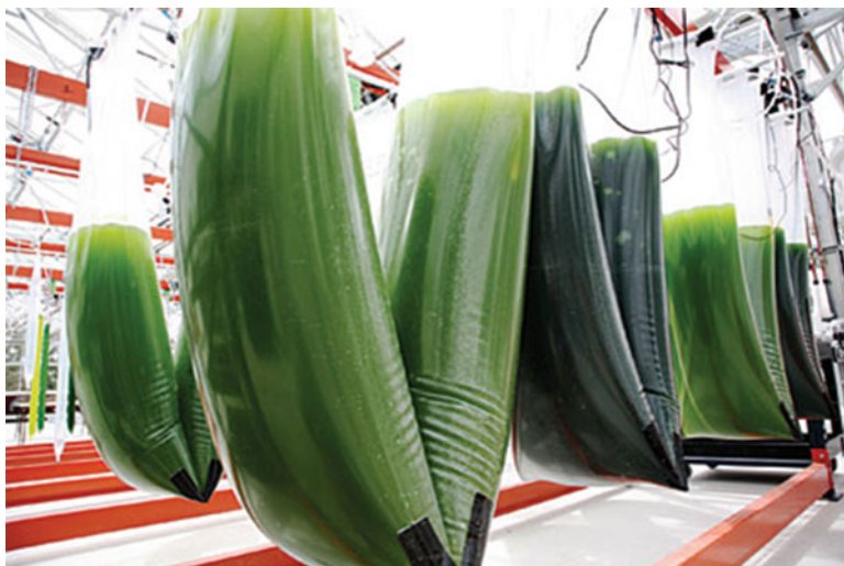
Fig. 8 Plastic sleeves (a) and plastic bags (b) as most simple systems for closed algal cultivation (online resource 4; with kind permission of Oilseed Crops )
