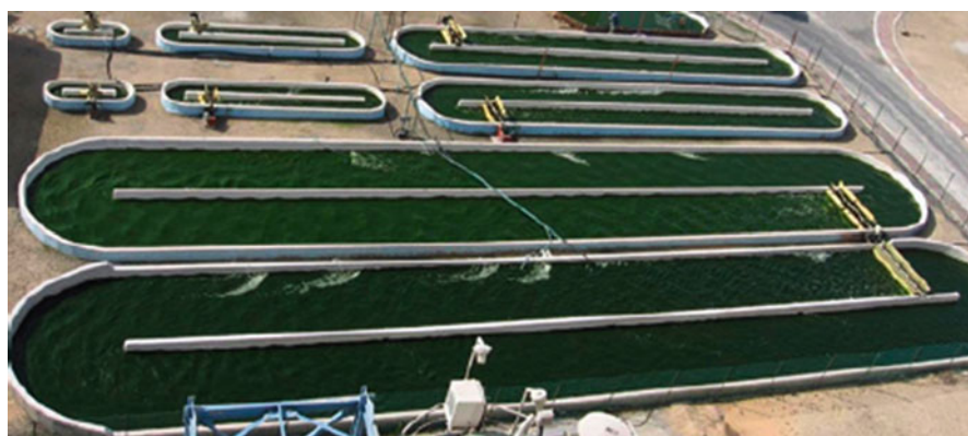
Fig. 2 Raceway pond with paddle wheels operated in outdoor mode. Different sizes of the ponds are used to prepare the inoculum cultures for the subsequent cultivation stage (online resource 2) (with permission of Algae Energy , UK)
