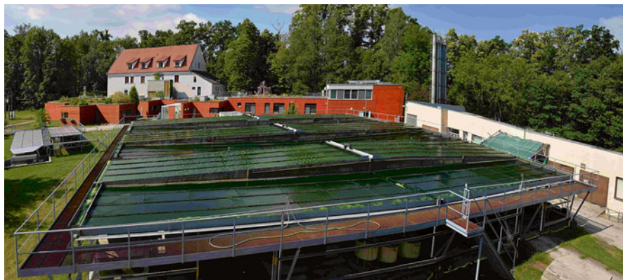
Fig. 6 Outdoor large-scale cascades of 650 m 2 with a working volume of 6,500 l built in the 1990s. Microalgae are grown in a smooth thin-layer of 6–8 mm and the total surface-to-volume ratio is about 100 m -1
