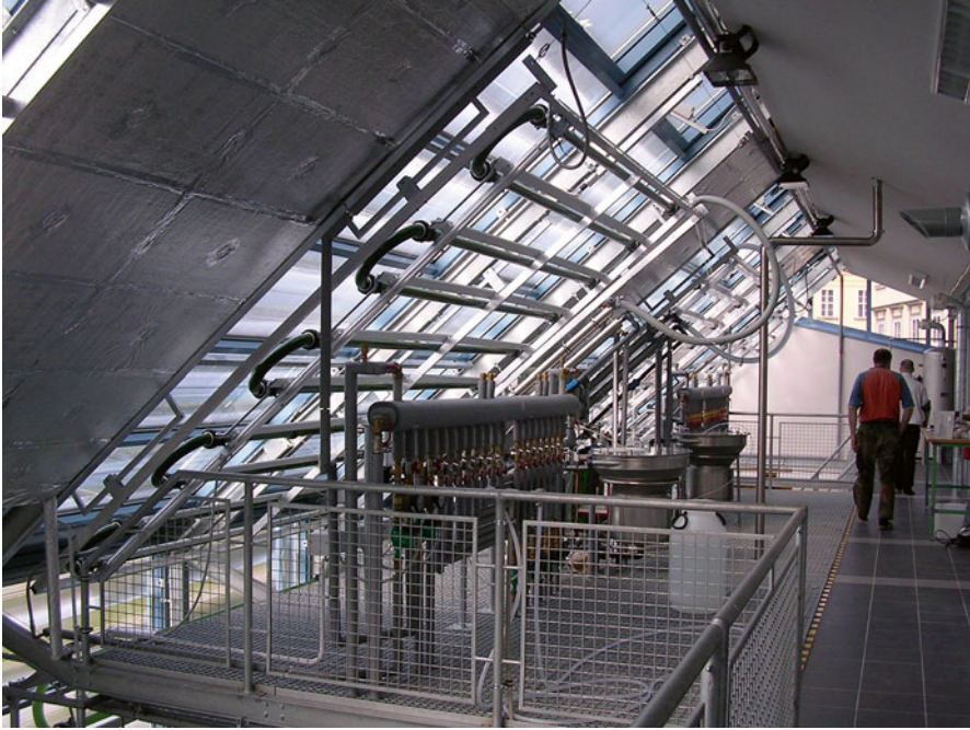
Fig. 1 An indoor PBR with a total volume of 120 L based uniquely on solar concentrators – linear Fresnel lenses. It was mounted in a greenhouse in the biotechnology hall of the Institute of Physical Biology, University of South Bohemia in Nové Hradý, Czech Republic. The tubular loop of the PBR was automatically kept in the focus of the solar concentrators which allowed for a maximum value of up to 6000 \mu\text{E m}^{-2} \text{s}^{-1} on the tube surface. This dual purpose system was designed for microalgae cultivation in temperate climate zone and with surplus heat being used for warming service water
