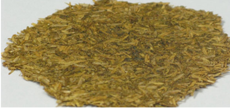
Fig. 8 Composite made with rice husks similar to conventional particleboard
