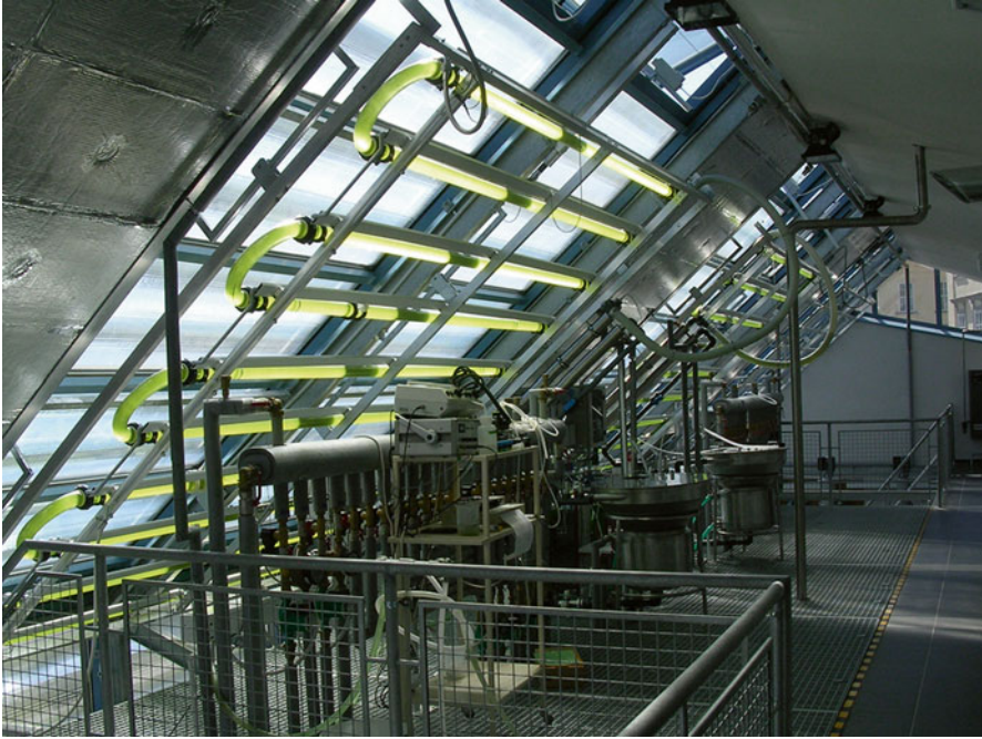
Fig. 7 Tubular serpentine photobioreactor based on solar concentrators – linear Fresnel lenses developed at the Center for Biotechnology, University of South Bohemia, Nové Hradky (Czech Republic) (Courtesy of Prof. J. Masojídek)
