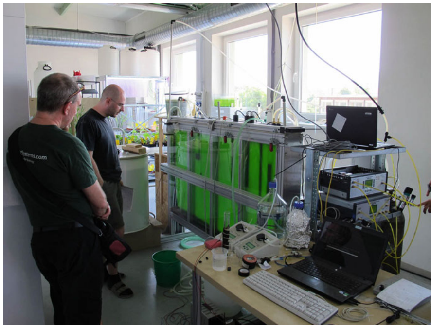
Fig. 17 120 L module unit of the Photon System Instruments (PSI) PBR (with kind permission by Photon System Instruments, spol. s.r.o., Czech Republic )
