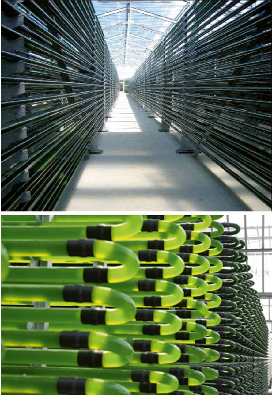
Fig. 6 Tubular manifold photobioreactors installed at Roquette Klötze & Co. KG (Germany) (Photo ©: Jörg Ullmann (Courtesy of J. Ullmann))
