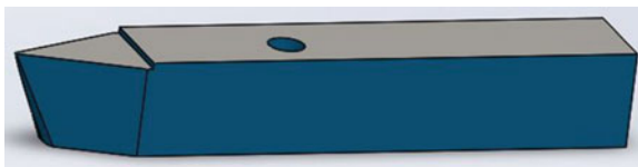
Fig. 9.14 Solid view of the V cutting tool (Design 2)
