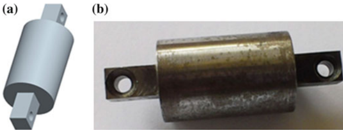
Fig. 6.9 a CAD model of roller bearing, b fabricated roller bearing
