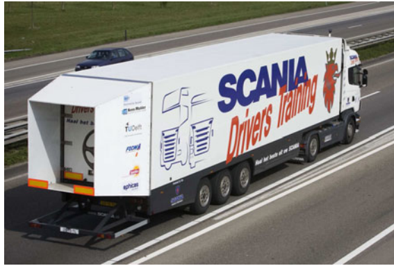
Fig. 11 Road test with the boat tail
