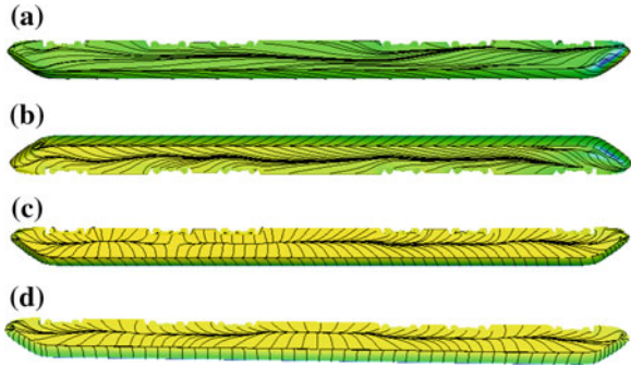
Fig. 15 Surface streamline patterns on the leeward side for different yaw angles. The flow direction is from right to left . a \beta = 20^\circ . b \beta = 50^\circ . c \beta = 80^\circ . d \beta = 90^\circ
