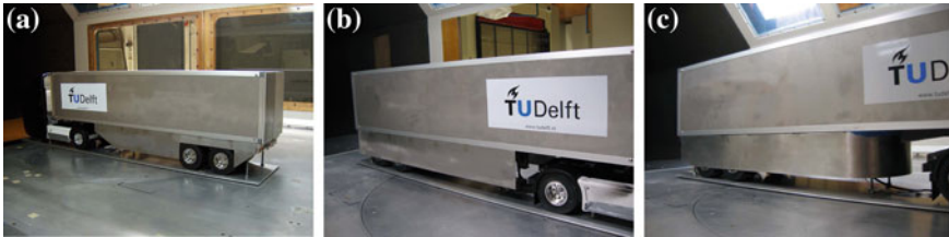
Fig. 6 Aerodynamic add-ons tested in the wind tunnel. a Skirt with uncovered wheels, b skirt with sharp front edge, c round enclosed skirt
