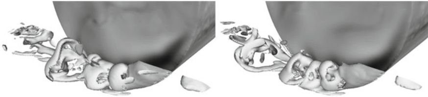
Fig. 3 Case 2. Jetting vortex on the inner side of the wheel. Iso-surface of second invariant of the velocity gradient tensor Q = 6 \times 10^6 . The time difference between the two pictures is t = 0.5 or tU_\infty/D = 0.196 , where D is diameter of the wheel
