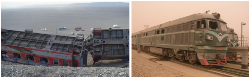
Fig. 1 Train overturned (left) and badly damaged (right) on the Lan-Xin railway
