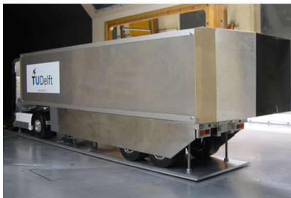
Fig. 13 Semi-trailer equipped with SideWings and a boat tail
