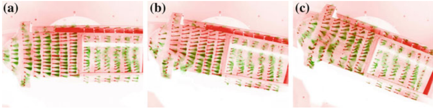
Fig. 4 Tufts on model (insight through plexiglas window): color coded picture from time series recording. a \alpha = 0^\circ , b \alpha = 10^\circ , c \alpha = 20^\circ
