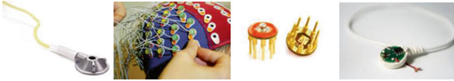
Fig. 5.1 EEG electrodes. From left to right, (1) conventional EEG electrode filled with conductive gel, (2) 64 electrode cap used at UOP-NU, (3) comb-like dry-contact electrode, (4) active electrode
