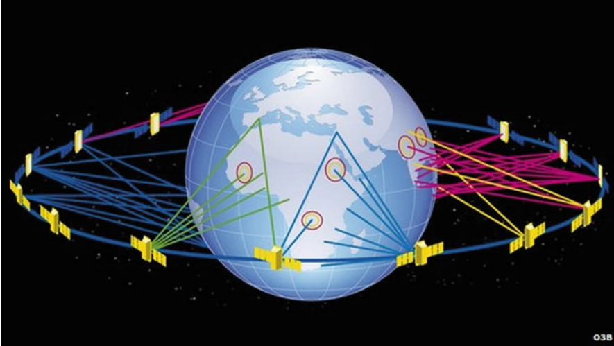
Fig. 6.4 The O3b satellite network that is optimized for Internet connectivity, lower latency, and low-cost service to the equatorial regions. (Graphic courtesy of O3b.)
