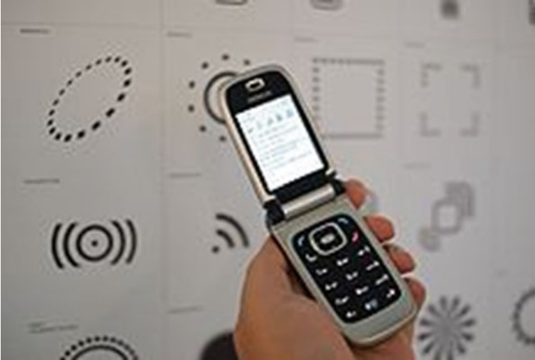
Fig. 5.2 An NFC-enabled mobile phone interacting with a smart poster
