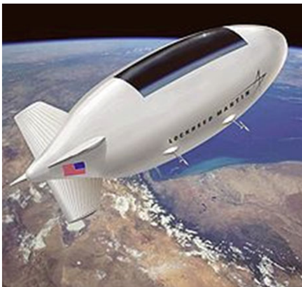
Fig. 6.2 An experimental airship conceived to support high altitude platform system (HAPS) services
