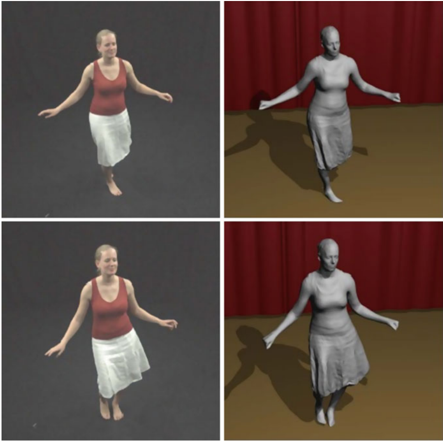
Fig. 5.2 de Aguiar et al. [10] started with a laser scan and found its deformation from eight video recordings
