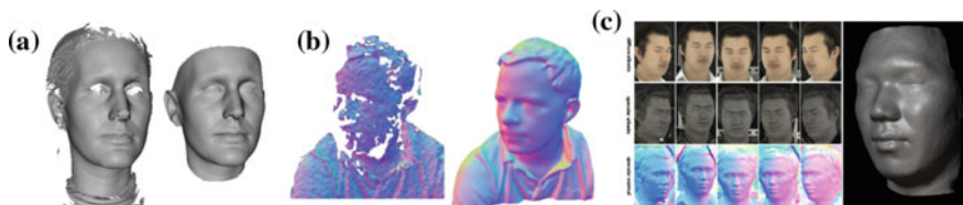
Fig. 6.3 Facial data acquisition methods: a data from a laser scanner [4]: raw data ( left ) and pre-processed data ( right ), b data from KinectFusion [15]: initial data ( left ) and accumulated data ( right ), c data from stereo images [14]: intrinsic images ( left ) and reconstructed model ( right )
