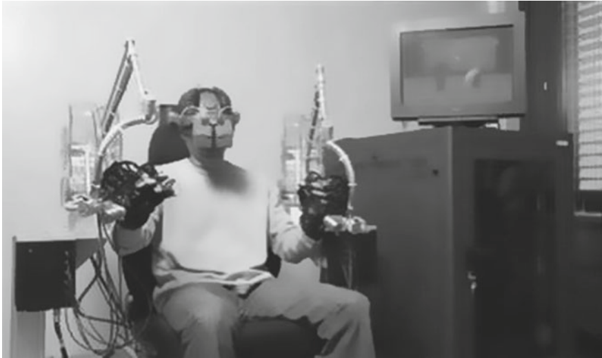
Fig. 9.2 Haptic workstation for two-handed manipulation [28]
