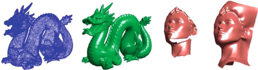
Fig. 5.1 Surface fitting by function reconstruction [4]
