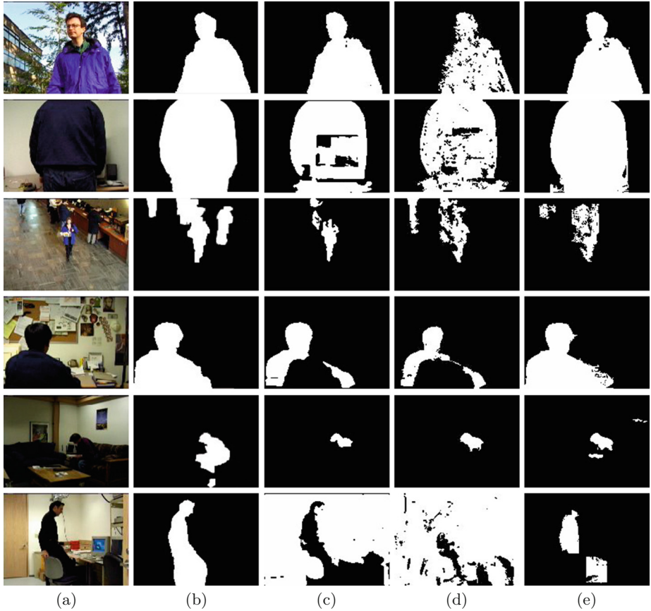
Fig. 2. (a) Original frames from video sequences, (b) Ground truth, (c) Results of method proposed by Stauffer and Grimson [2], (d) Results of hybrid method proposed by M. Haque et al. [5], and (e) Results of proposed method
